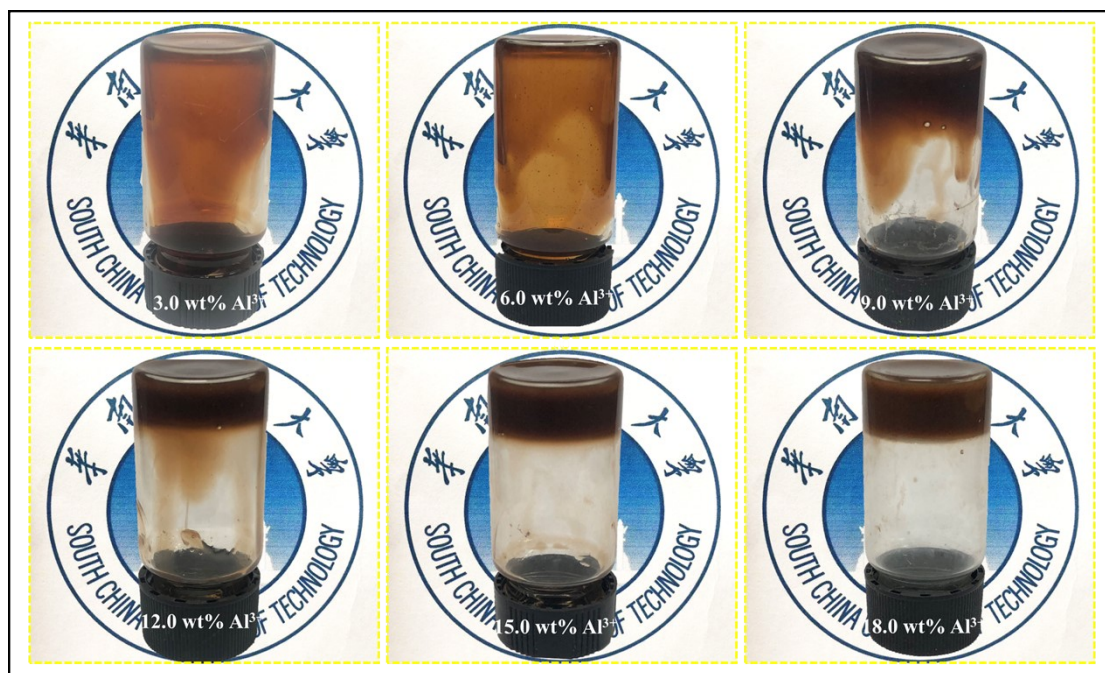
Figure. S3 Various hydrogels from different \text{Al}^{3+} contents (28.0 wt% AA, 0.25 wt% APS, and 0.6 wt% DESL).
