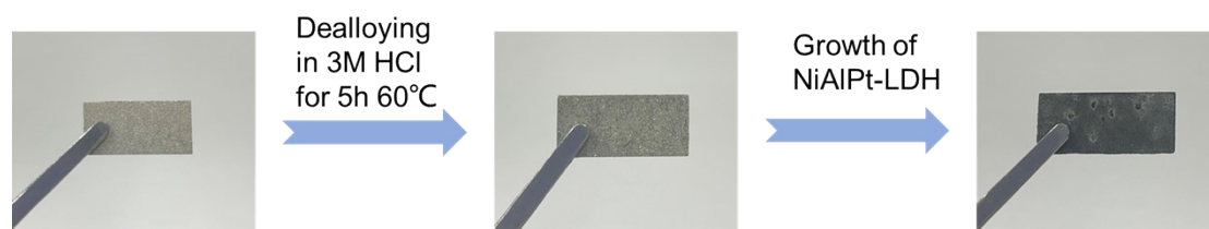
Figure S1. Digital photographs of EHEA, PHEA and NiAlPt-LDH@PHEA, respectively. As shown in the figure, the eutectic high-entropy alloy has a bright metallic luster. After acid dealloying, the color becomes darker and the thickness becomes thinner. The surface modified HEA-based electrode shows a light blue state, indicating the successful growth of LDH.
