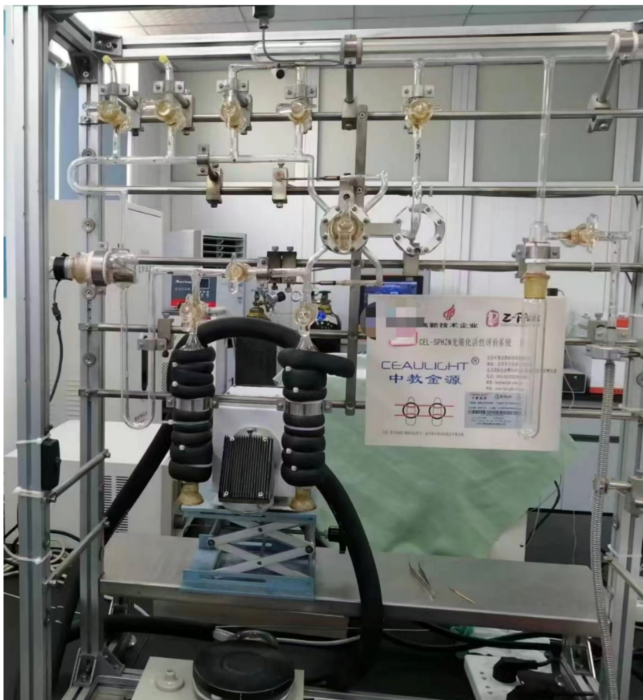
Fig. S1 The CEL-SPH2N-D9 automatic photocatalytic activity evaluation system.
