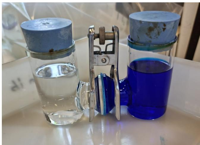
Figure S6. Home-built VO<sup>2+</sup> diffusion cell.
