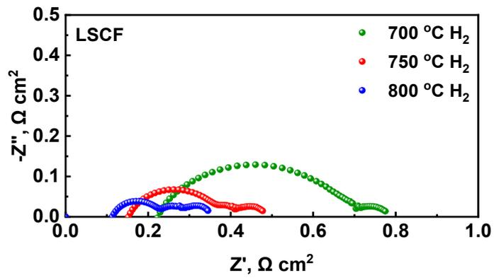
Figure S3. EIS of a single cell with the LSCF cathode, measured at 700-800 °C.
