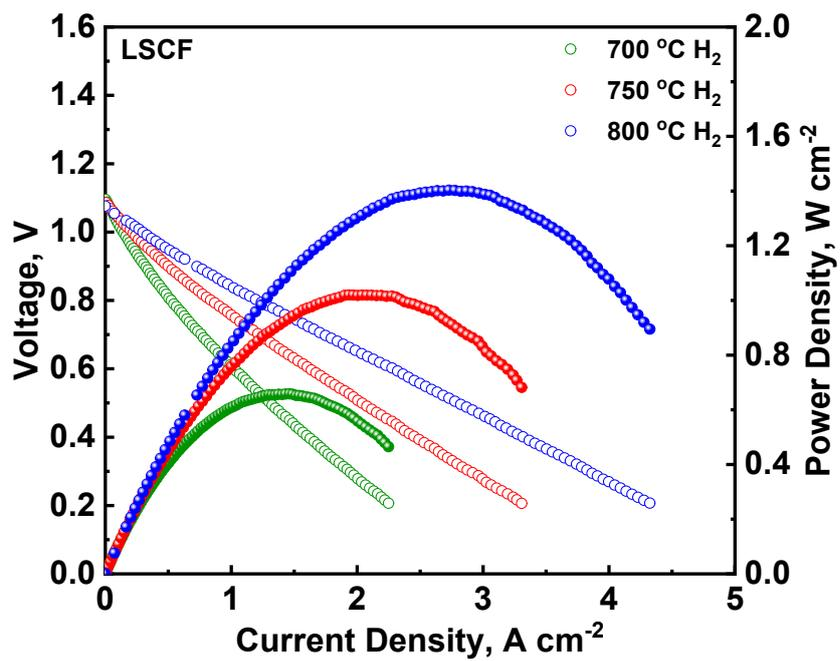
Figure S2. Typical I-V-P curves of single cell with the LSCF cathode, measured in FC mode at 700-800 °C.
