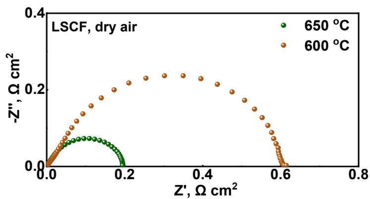
Figure S1. EIS of symmetrical cells with the LSCF electrode tested at 600-800 °C in the air.
