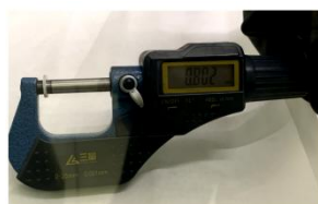
Figure S5. Thickness of 110 mg LPSC (100 mg) -PTFE (10 mg) layer.
