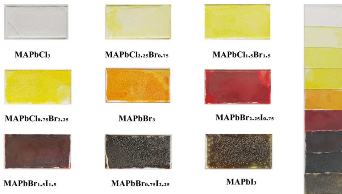
Figure S13. 9 kinds of MAPbX 3 type perovskites. Perovskite solution is spun onto a glass plate, and the solvent is steamed to take pictures.
