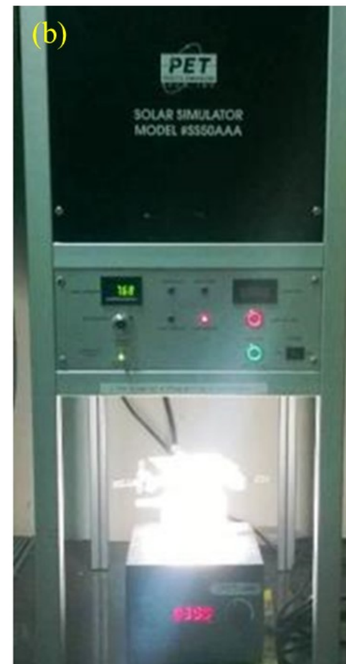
Figure S2. (a) A schematic photocatalytic reactor set-up. (b) Photocatalytic reactor system in a solar simulator.
