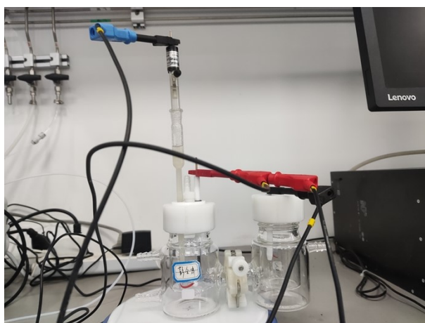
Figure S14. The typical H-type electrochemical cell separated by a Nafion 117 membrane.
