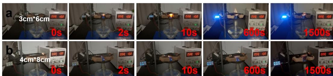
**Fig. S9** The fire warning process snapshots of different-sized  $P_1G_1P_{0.8}$  nanocomposite film under fire attack.
