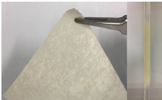
Figure S3. The photograph of flexible P(VEC-SF)-PE film with tunable size.
