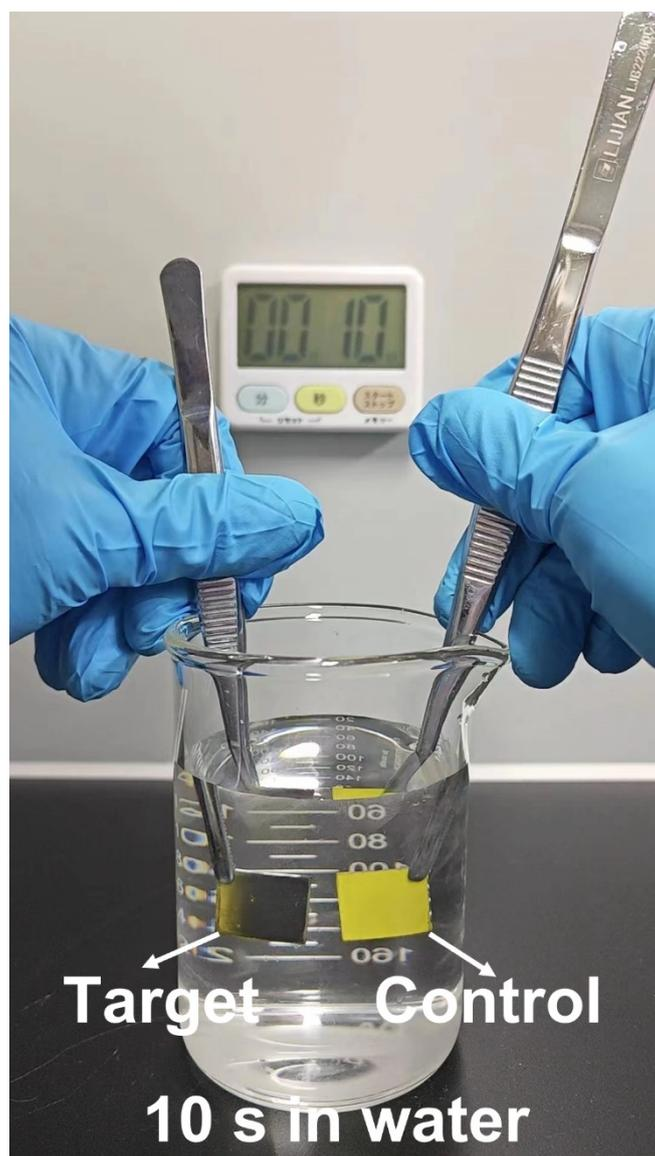
**Figure S23.** Photograph of the control and target perovskite films dipped in water.
