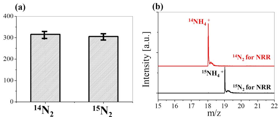
**Figure S7.** (a)  $^{15}\text{N}_2$  isotope labelling experiment for the NRR, (b) MALDI-MS spectra for the qualitative isotope labelling test.
