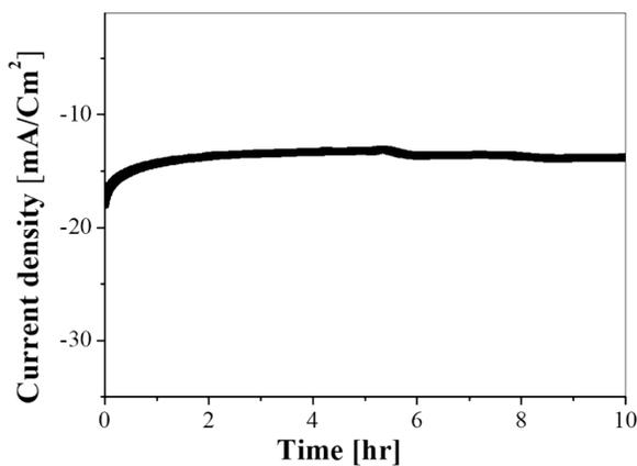
**Figure S8.** Plot depicting the current-time profile of the PtRu@TiN/NG electrode, recorded at -1 V in an  $\text{N}_2$  environment with light exposure for a duration of 10 hours.
