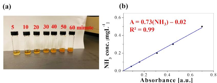
**Figure S2.** (a) Reaction product collection using Nessler reagent from PtRu@TiN/NG, (b) calibration curve used for estimation of  $\text{NH}_3$  concentration. The absorbance at 420 nm was measured by UV-vis spectrophotometer.
