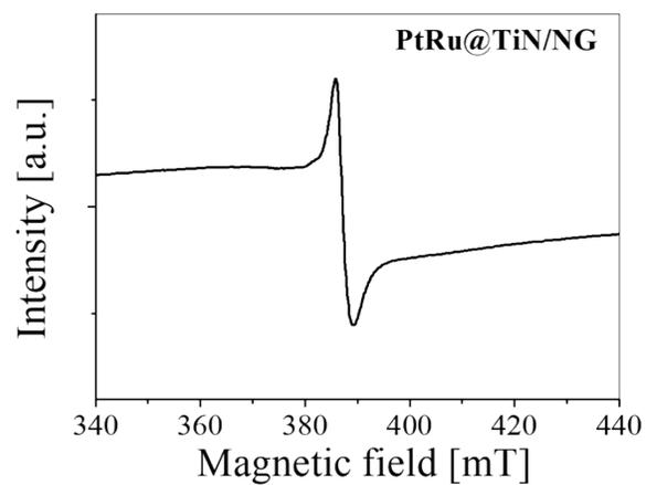
**Figure S4.** EPR spectra of PtRu@TiN/NG sample at room temperature.
