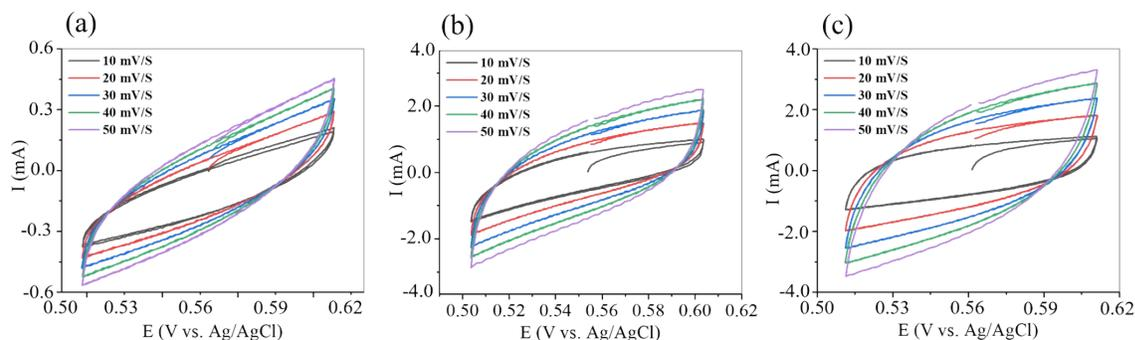
**Figure S9.** Effective electrochemical active surface area tests (ECSA) of (a) PtRu@TiN, (b) PtRu@NG, and (c) PtRu@NG.
