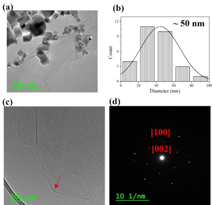
**Figure S3.** TEM image of (a-b) TiN NPs and its histogram illustrating the size distribution (c) pure monolayer N doped graphene i.e., NG indicated by arrow, (d) corresponding SAED pattern.
