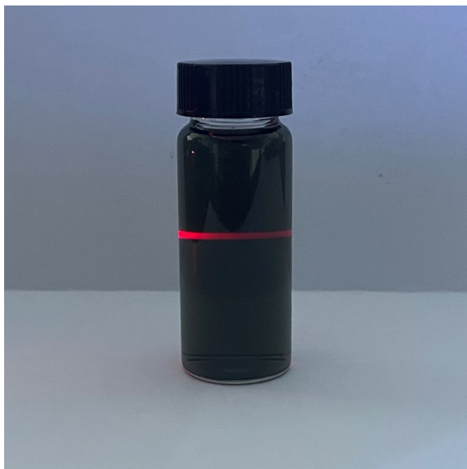
Figure S2 The Tyndall effect of \text{Ti}_3\text{C}_2\text{T}_x suspension.
