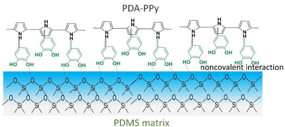
**Fig. S2** Schematic diagram of adhesion between PDA-PPy and PDMS matrix
