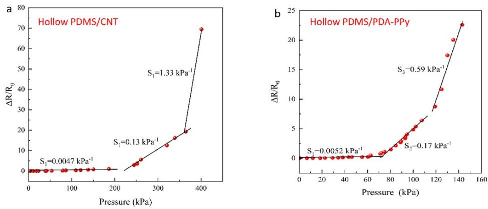
**Fig. S12** Pressure sensitivities of the sensors based on the hollow PDMS/CNT and PDMS/PDA-PPy
