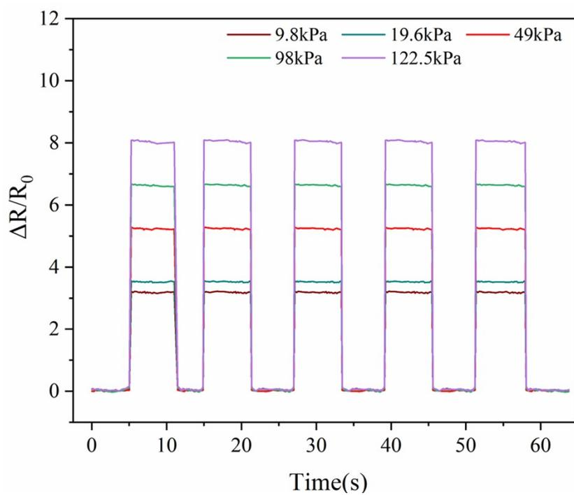
**Fig. S10** Relative resistance response to different cyclic external forces
