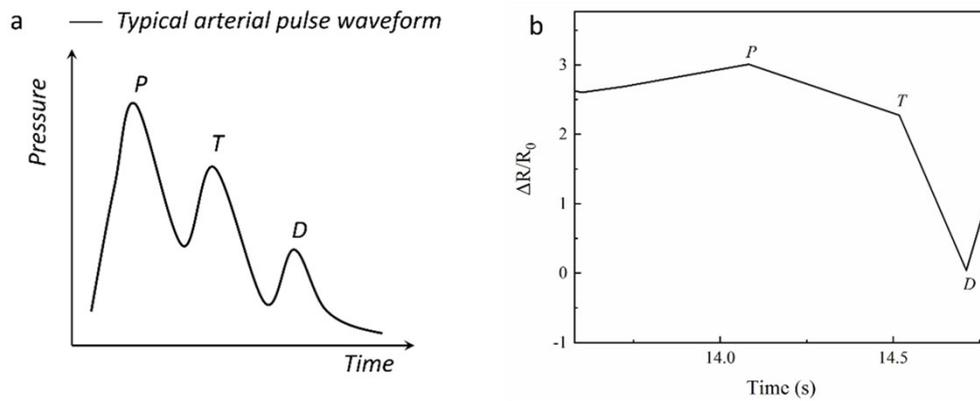
**Fig. S6** a) Typical arterial pulse waveform with P, T and D peaks. b) Change in relative resistance of arterial pulse waveform by sticking the sensor to the wrist artery
