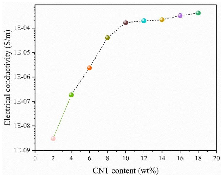
**Fig. S1** The conductivity of the hollow PDMS/CNT composite as a function of CNT contents
