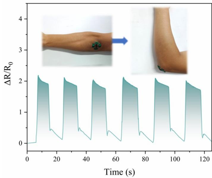
**Fig. S8** Relative resistance response to detecting the elbow bending
