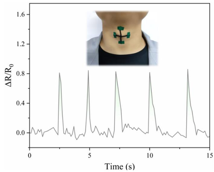
**Fig. S7** Relative resistance response to detecting the swallowing action
