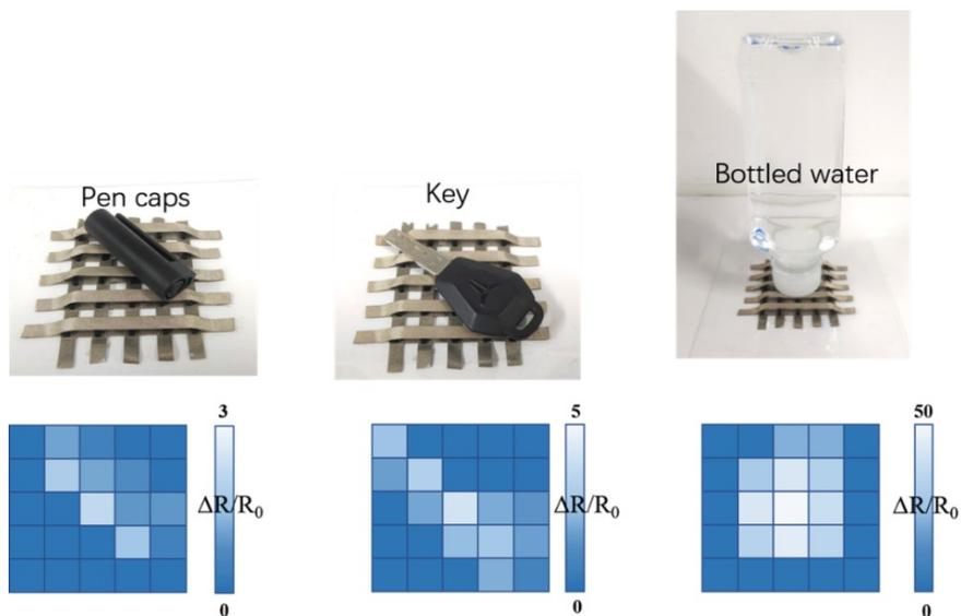
**Fig. S9** Different objects applied to the sensor array and their pressure mapping
