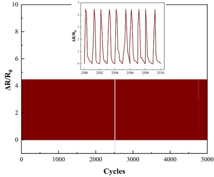
**Fig. S11.** Relative resistance change of the pressure sensor under 500 cycles of loading and unloading the 300 kPa pressure
