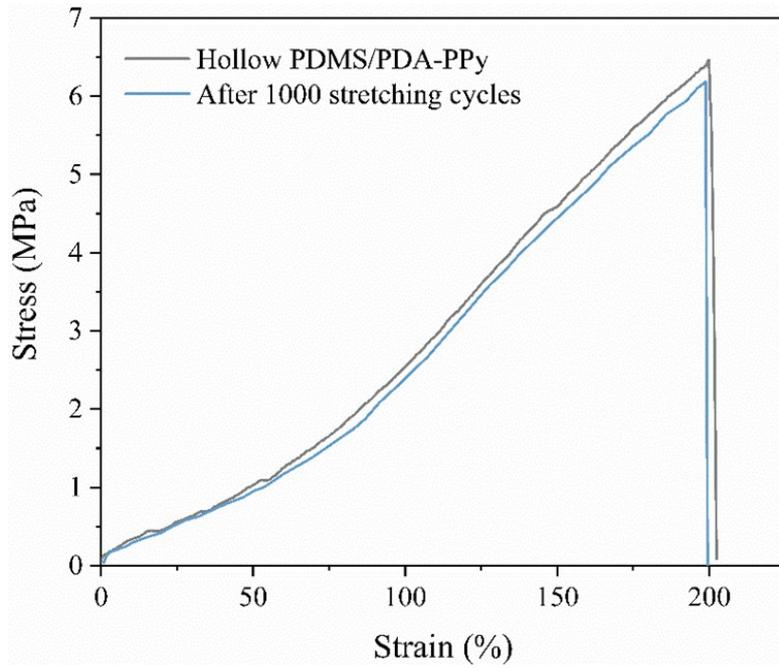
**Fig. S5** Stress-strain curves of hollow PDMS/PDA-PPy fiber and its curve after 1000 stretching cycles
