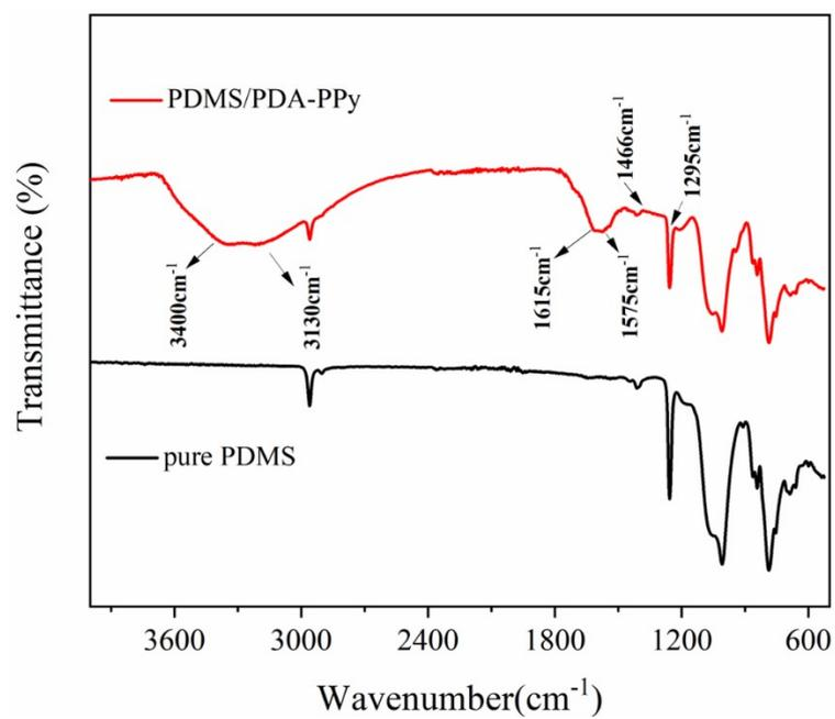
**Fig. S3** FTIR spectra of the pure PDMS fiber and PDMS/PDA-PPy composite fiber
