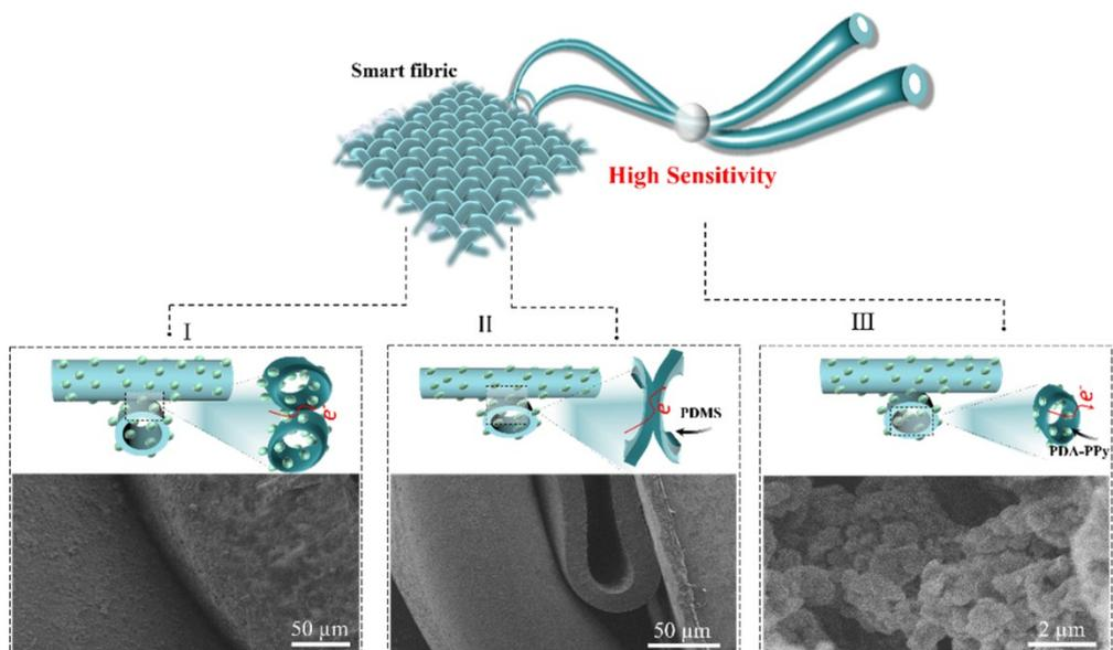
**Fig. S13** Schematic diagram and SEM images of the morphology changes of the sensor under continuous external force
