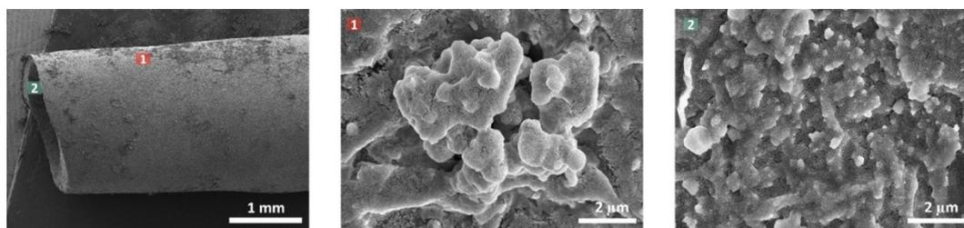
**Fig. S4** SEM morphology of the outer and inner surfaces of the PDMS/PDA-PPy composite fiber
