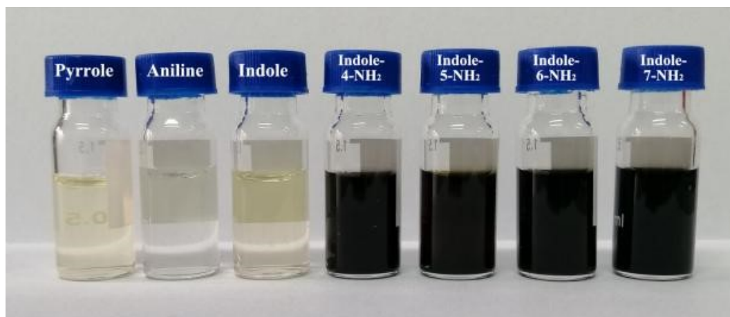
Fig. S1 Photographs of the conductive polymers prepared under acidic system with \text{pH} = 3.0 and ammonium persulfate as the oxidant. The only difference from the preparation of hydrogels is that no PEDOT:PSS solution was added during this process.
