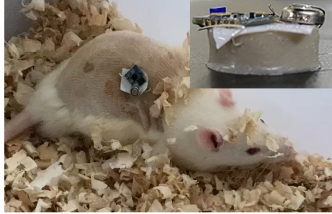
Fig. S6 Photographs of assembled PPA-Ag hydrogel matrix with real-time and remote monitoring module on a rat wound healing.
