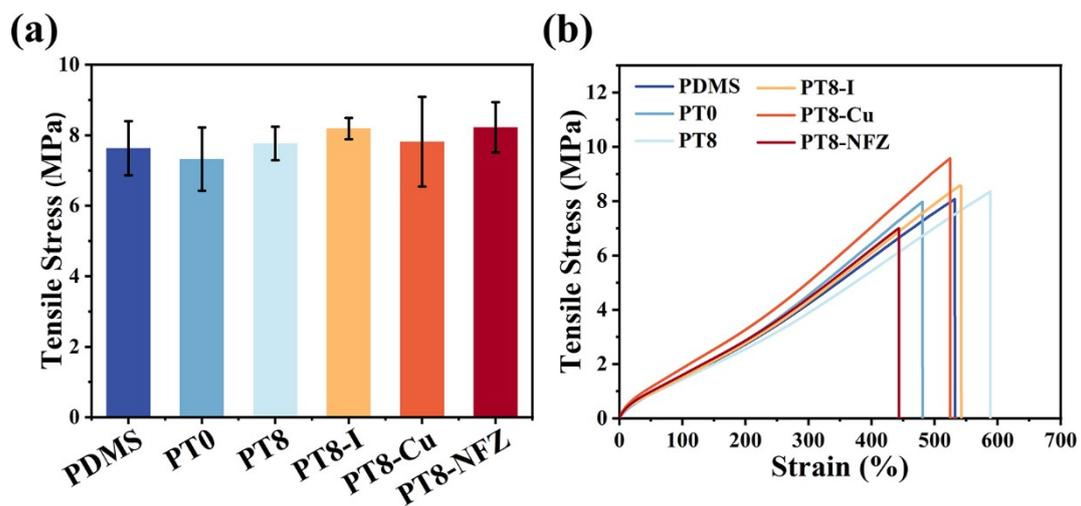
**Figure S1.** (a) Tensile strength of pristine PDMS and modified PDMS. (b)
