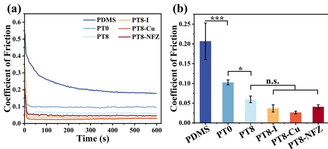
**Figure S2.** (a) COF-time curves of pristine PDMS surface and modified PDMS surfaces in artificial urine. (b) The average values of COF of pristine PDMS and modified PDMS in artificial urine.
