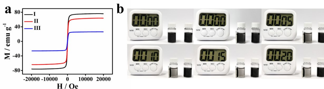
Fig. S5. (a) The magnetic hysteresis loops of \text{Fe}_3\text{O}_4 (I), \text{Fe}_3\text{O}_4@\text{TiO}_2 (II), and \text{Fe}_3\text{O}_4@\text{TiO}_2@\text{MoS}_2 (III) and (b) physical drawing of magnetic separation of \text{Fe}_3\text{O}_4@\text{TiO}_2@\text{MoS}_2 .
