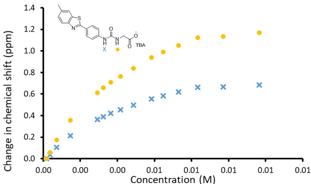
Figure S31 - Graph illustrating the  $^1\text{H}$  NMR down-field change in chemical shift of urea NH resonances with increasing concentrations of SSA **6** in  $\text{DMSO-}d_6$  0.5 %  $\text{H}_2\text{O}$  solution (298 K).
