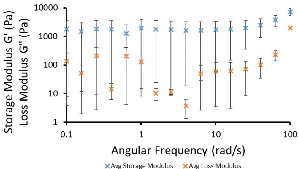
Figure S105 - Graph showing average results (n=3) from frequency sweep experiments obtained from the linear viscoelastic region under a constant shear strain ( $\gamma$ ) of 0.0720 % (298 K). SSA 7 (5 mg) in 1 mL of aqueous NaOBz solution (0.505 M). Error = standard deviation of the mean.
