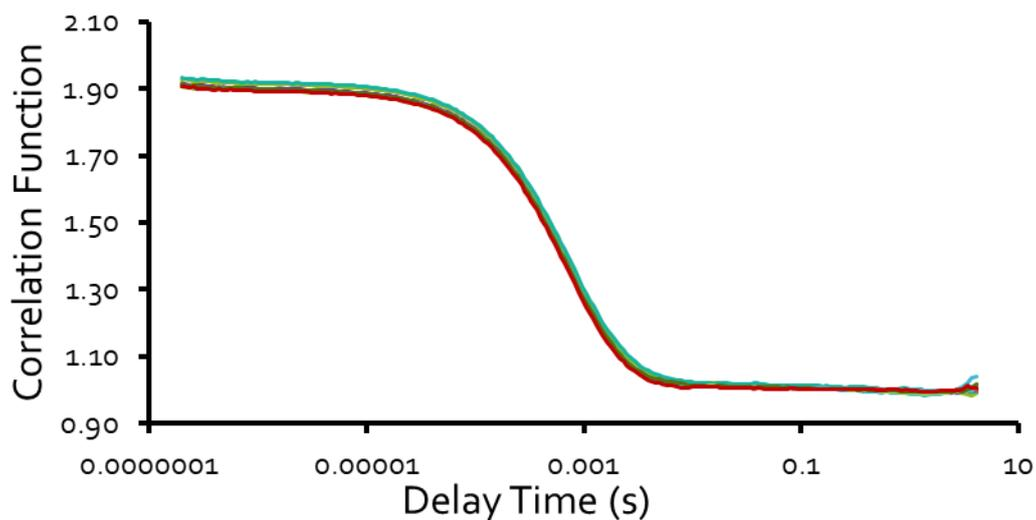
Figure S56 – Correlation function data for 10 DLS runs of SSA 7 (0.56 mM) in an EtOH:H<sub>2</sub>O (1:19) solution at 298 K.
