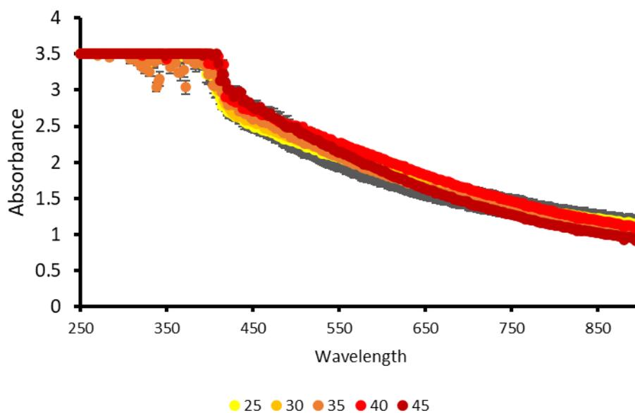
Figure S159 - Average (n=3) absorbance graph of **4** (1.5 mg/mL) in NaOBz recorded for each 200  $\mu$ L sample at 5-degree increments from 25-45  $^{\circ}$ C. Error = standard deviation of the mean.
