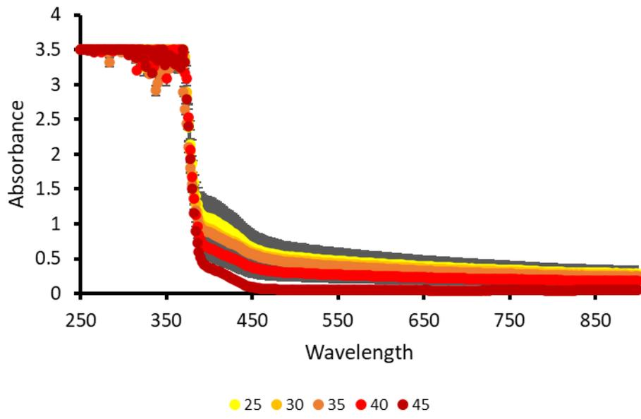
Figure S158 - Average (n=3) absorbance graph of **4** (1.5 mg/mL) in NaH<sub>2</sub>PO<sub>4</sub> recorded for each 200  $\mu$ L sample at 5-degree increments from 25-45  $^{\circ}$ C. Error = standard deviation of the mean.
