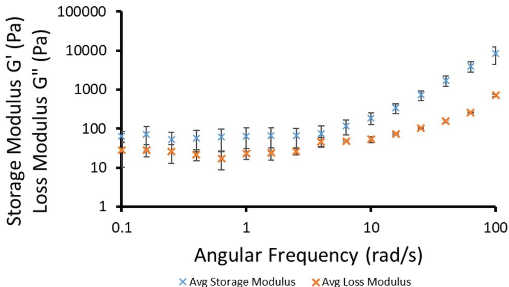
Figure S104 - Graph showing average results (n=3) from frequency sweep experiments obtained from the linear viscoelastic region under a constant shear strain ( $\gamma$ ) of 0.0195 % (298 K). SSA 7 (5 mg) in 1 mL of aqueous NaNO<sub>3</sub> solution (0.505 M). Error = standard deviation of the mean.
