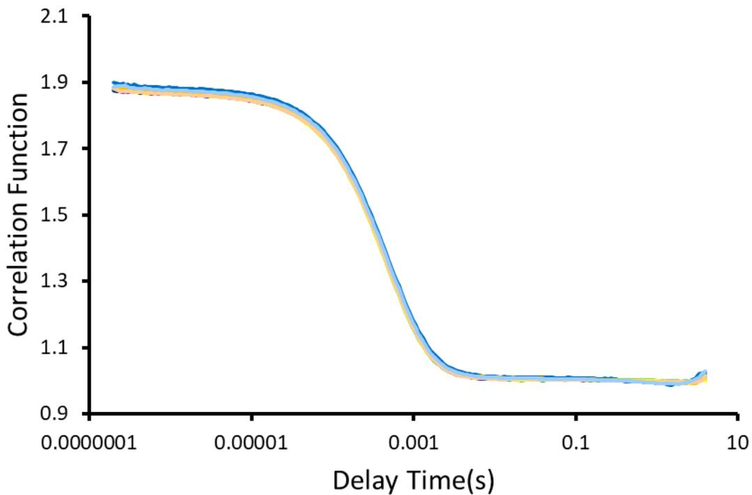
Figure S48 - Correlation function data for 10 DLS runs of SSA 4 (0.56 mM) in an EtOH:H<sub>2</sub>O (1:19) solution at 298 K.
