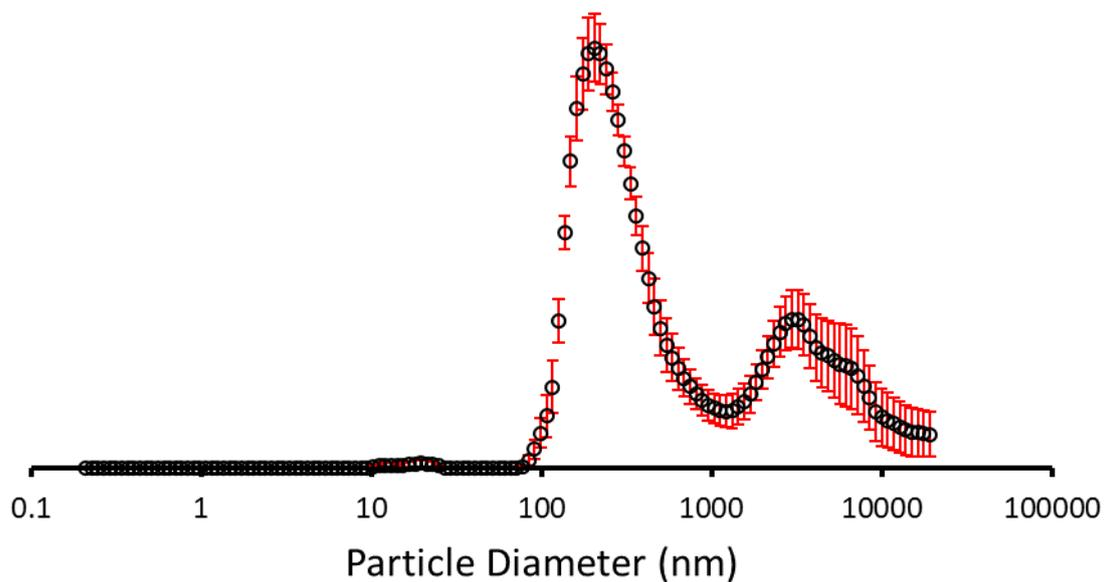
Figure S53 - The average intensity particle size distribution calculated (790 nm) using 10 DLS runs for SSA **6** (0.28 mM) in an EtOH:H<sub>2</sub>O (1:19) solution at 298 K.
