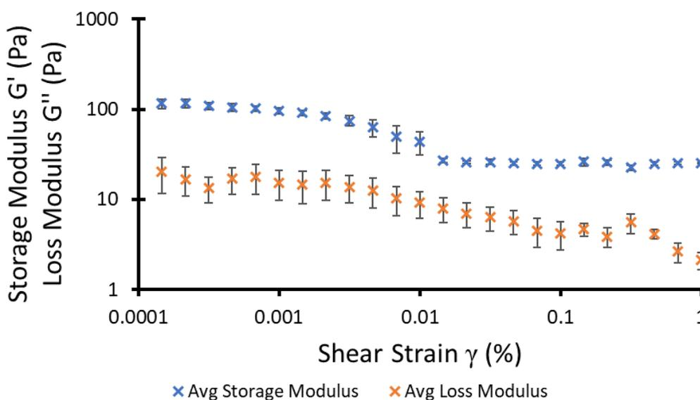
Figure S99 - Graph showing average results ( $n=3$ ) from amplitude sweep experiments used to define the linear viscoelastic region of the sample at 298 K. SSA 7 (5 mg) in 1 mL of aqueous NaNO<sub>3</sub> solution (0.505 M) (1 = 100 %). Error = standard deviation of the mean.
