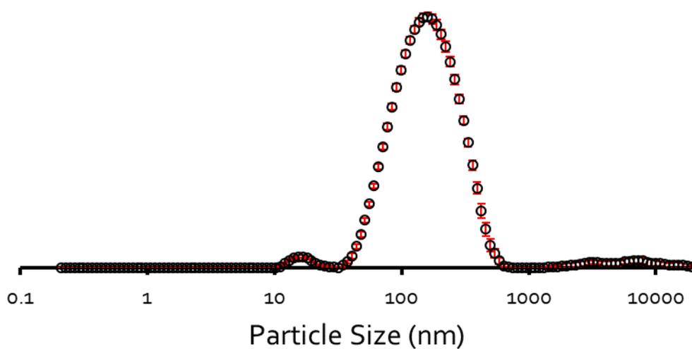
Figure S57 – The average intensity particle size distribution calculated (153 nm) using 10 DLS runs for SSA 7 (0.56 mM) in an EtOH:H<sub>2</sub>O (1:19) solution at 298 K.
