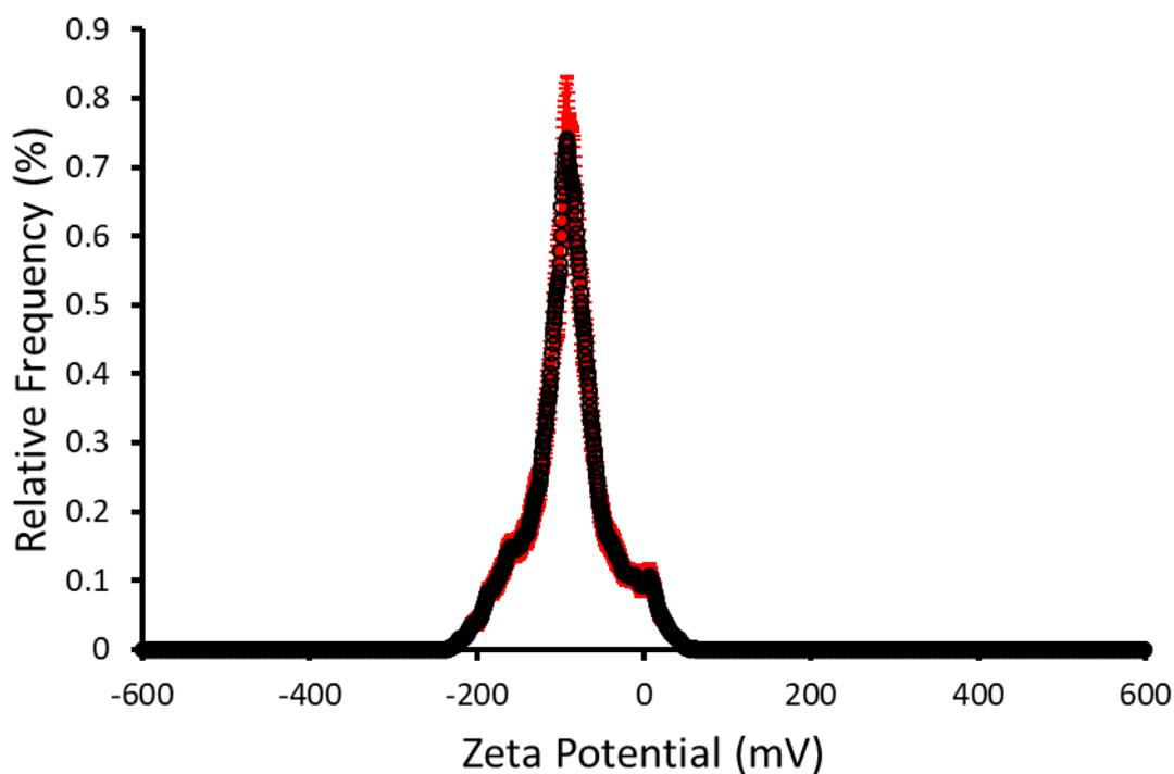
Figure S61 - The average zeta potential distribution calculated using 10 runs for SSA 3 (5.56 mM) in EtOH:H<sub>2</sub>O (1:19) solution at 298 K. Average measurement value -88.29 mV.
