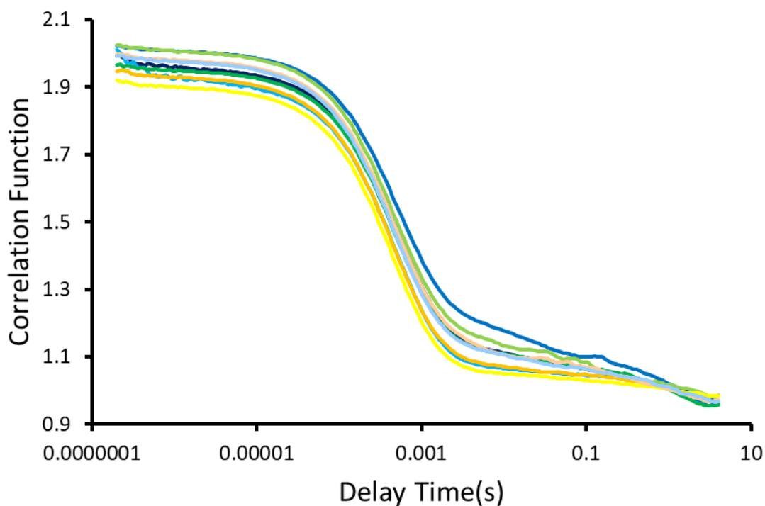
Figure S50 - Correlation function data for 10 DLS runs of SSA **6** (2.78 mM) in an EtOH:H<sub>2</sub>O (1:19) solution at 298 K.
