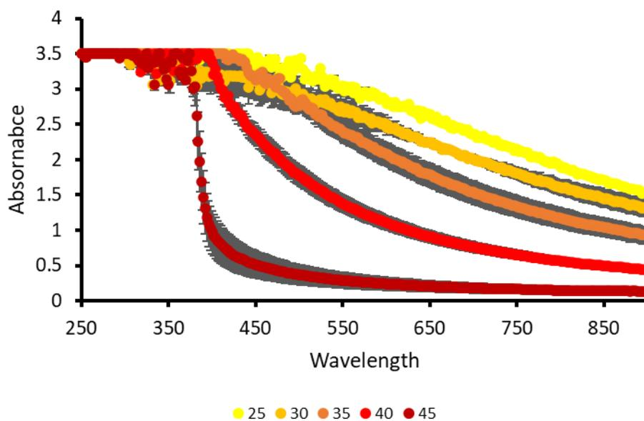
Figure S147 - Average (n=3) absorbance graph of **3** (1.5 mg/mL) in NaCl recorded for each 200  $\mu$ L sample at 5-degree increments from 25-45  $^{\circ}$ C. Error = standard deviation of the mean.
