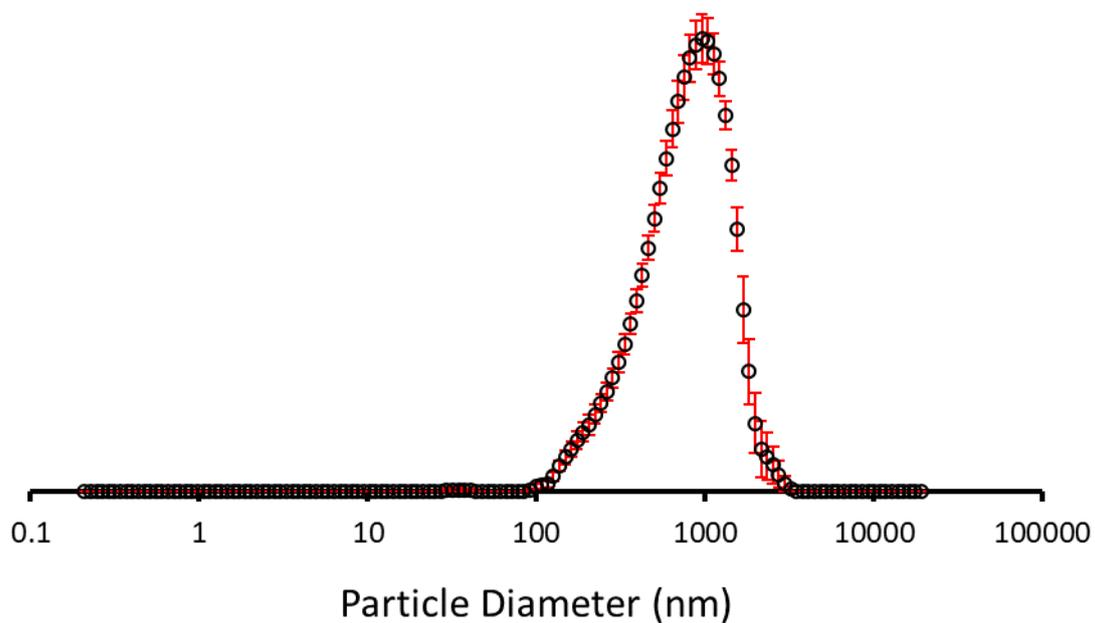
Figure S43 - The average intensity particle size distribution calculated (105 nm) using 10 DLS runs for SSA **3** (5.56 mM) in an EtOH:H<sub>2</sub>O (1:19) solution at 298 K.
