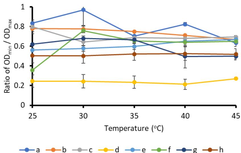
Figure S193 - Average (n=3) ratio values (OD<sub>495</sub> minimum/OD<sub>495</sub> maximum) taken from spectral well scan data of **4** (1.5 mg/mL). Error bars represent the full range of OD<sub>450</sub> ratio values to be calculated from the n=3 OD<sub>495</sub> maxima and minimum data. a = NaCl, b = KCl, c = NaNO<sub>3</sub> d = NaH<sub>2</sub>PO<sub>4</sub> e = NaOBz, f = DMSO, g = H<sub>2</sub>O.
