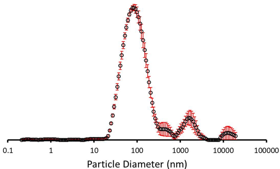
Figure S51 - The average intensity particle size distribution calculated (94 nm) using 10 DLS runs for SSA **6** (2.78 mM) in an EtOH:H<sub>2</sub>O (1:19) solution at 298 K.
