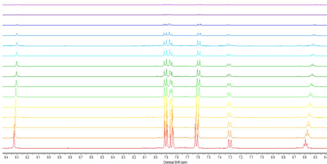
Figure S24 - Enlarged  $^1\text{H}$  NMR stack plot of SSA **3** in a  $\text{DMSO-}d_6$  0.5 %  $\text{H}_2\text{O}$  solution. Samples were prepared in series with an aliquot of the most concentrated solution undergoing serial dilution.
