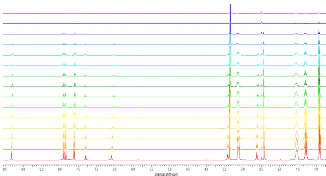
Figure S23 -  $^1\text{H}$  NMR stack plot of SSA **3** in a  $\text{DMSO-}d_6$  0.5 %  $\text{H}_2\text{O}$  solution. Samples were prepared in series with an aliquot of the most concentrated solution undergoing serial dilution.
