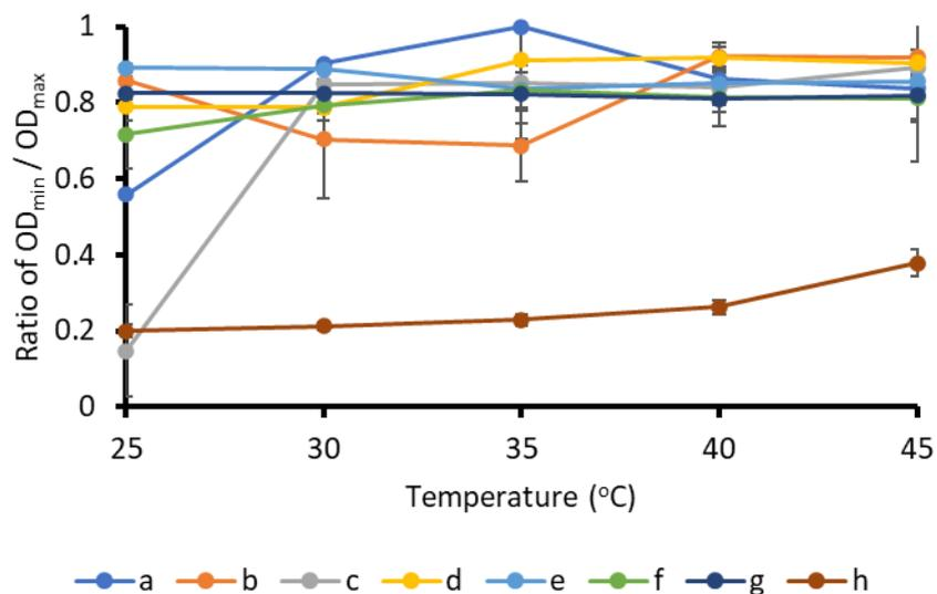
Figure S192 – Average (n=3) ratio values (OD<sub>495</sub> minimum/OD<sub>495</sub> maximum) taken from spectral well scan data of **3** (1.5 mg/mL). Error bars represent the full range of OD<sub>450</sub> ratio values to be calculated from the n=3 OD<sub>495</sub> maxima and minimum data. a = NaCl, b = KCl, c = NaNO<sub>3</sub> d = NaH<sub>2</sub>PO<sub>4</sub> e = NaOBz, f = DMSO, g = H<sub>2</sub>O.
