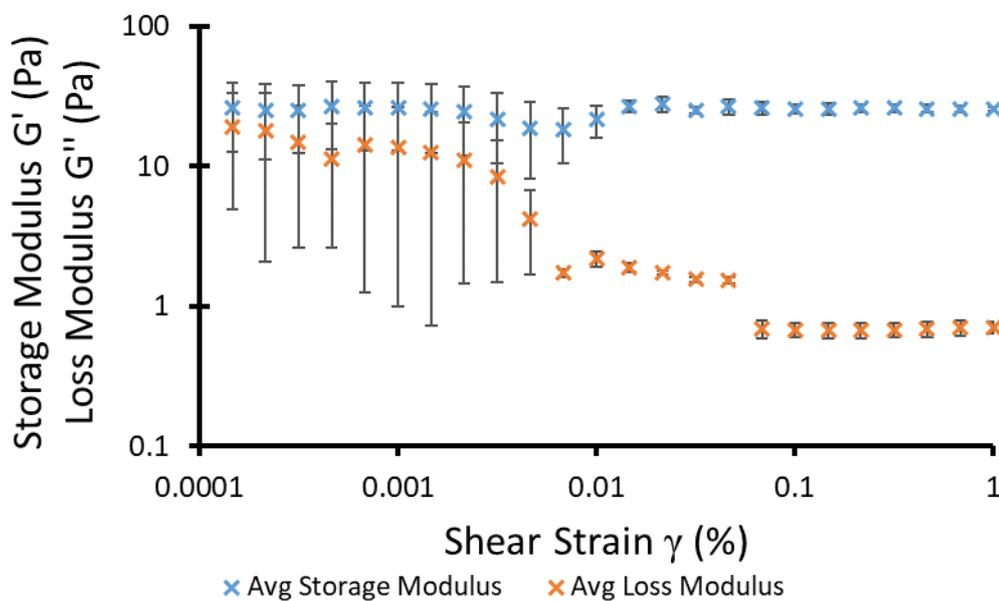
Figure S101 - Graph showing average results (n=3) from amplitude sweep experiments used to define the linear viscoelastic region of the sample at 298 K. SSA 7 (5 mg) in 1 mL of aqueous  $\text{NaOBz}$  solution (0.505 M) (1 = 100 %). Error = standard deviation of the mean.
