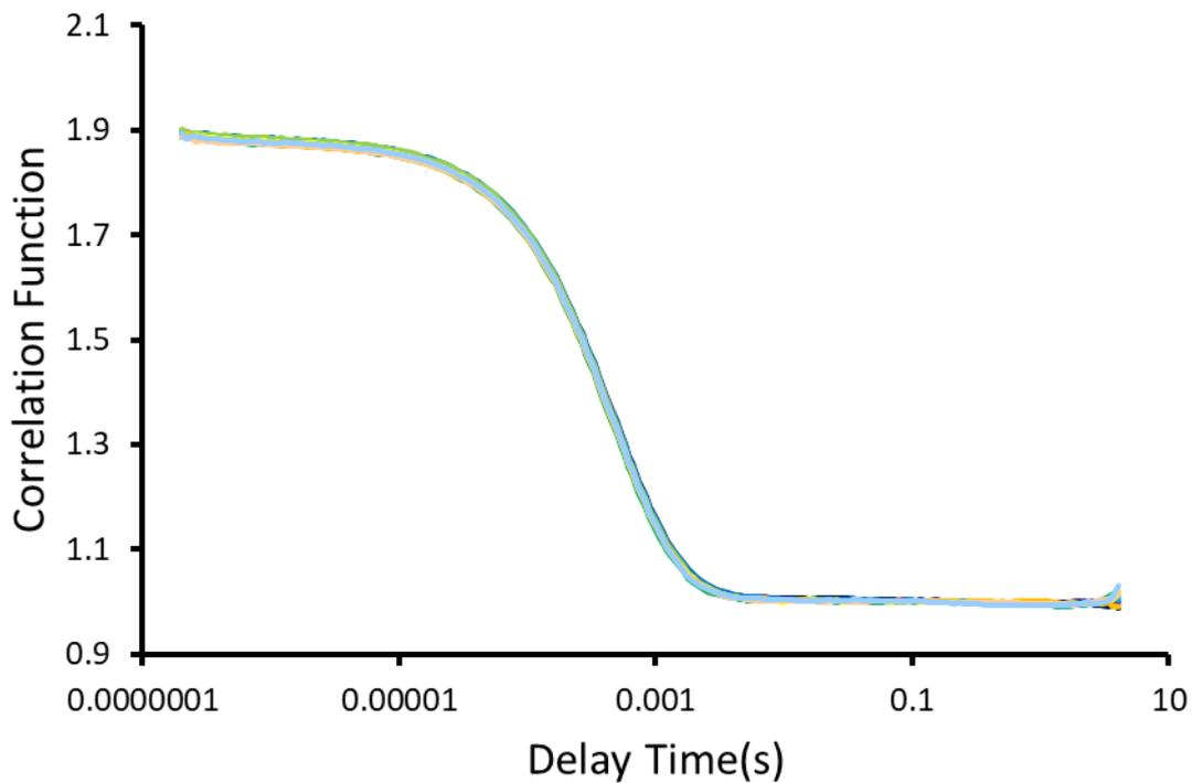
Figure S46 - Correlation function data for 10 DLS runs of SSA 4 (5.56 mM) in an EtOH:H<sub>2</sub>O (1:19) solution at 298 K.
