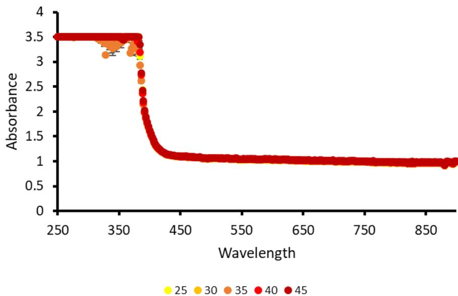
Figure S169 - Average (n=3) absorbance graph of **5** (1.5 mg/mL) in DMSO recorded for each 200  $\mu$ L sample at 5-degree increments from 25-45  $^{\circ}$ C. Error = standard deviation of the mean.
