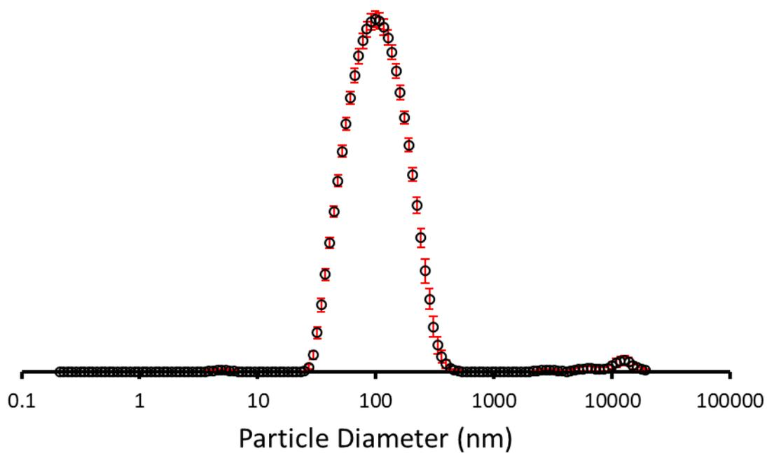
Figure S47 - The average intensity particle size distribution calculated (105 nm) using 10 DLS runs for SSA 4 (5.56 mM) in an EtOH:H<sub>2</sub>O (1:19) solution at 298 K.
