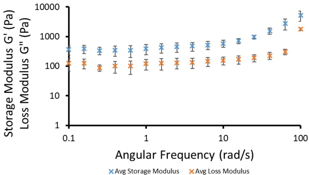
Figure S103 - Graph showing average results (n=3) from frequency sweep experiments obtained from the linear viscoelastic region under a constant shear strain ( $\gamma$ ) of 0.0277 % (298 K). SSA 7 (5 mg) in 1 mL of aqueous NaCl solution (0.505 M). Error = standard deviation of the mean.
