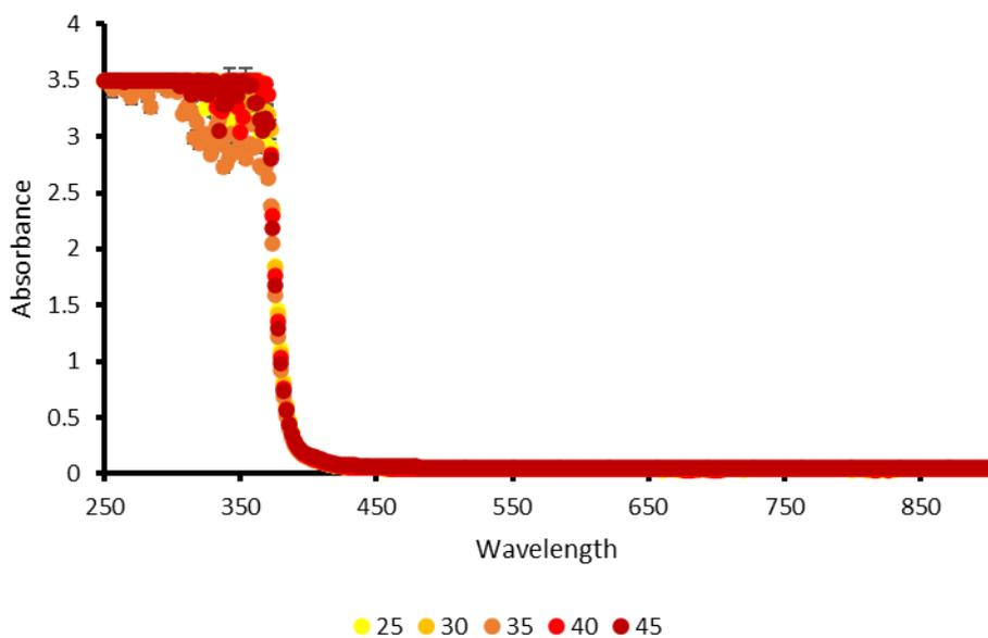
Figure S162 - Average (n=3) absorbance graph of **4** (1.5 mg/mL) in H<sub>2</sub>O recorded for each 200  $\mu$ L sample at 5-degree increments from 25-45  $^{\circ}$ C. Error = standard deviation of the mean.
