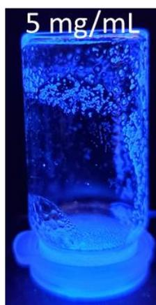
Figure S93 – SSA 7 MGC determination in 0.505 M aqueous  $\text{KCl}$ . Precipitation occurred so MGC could not be calculated.
