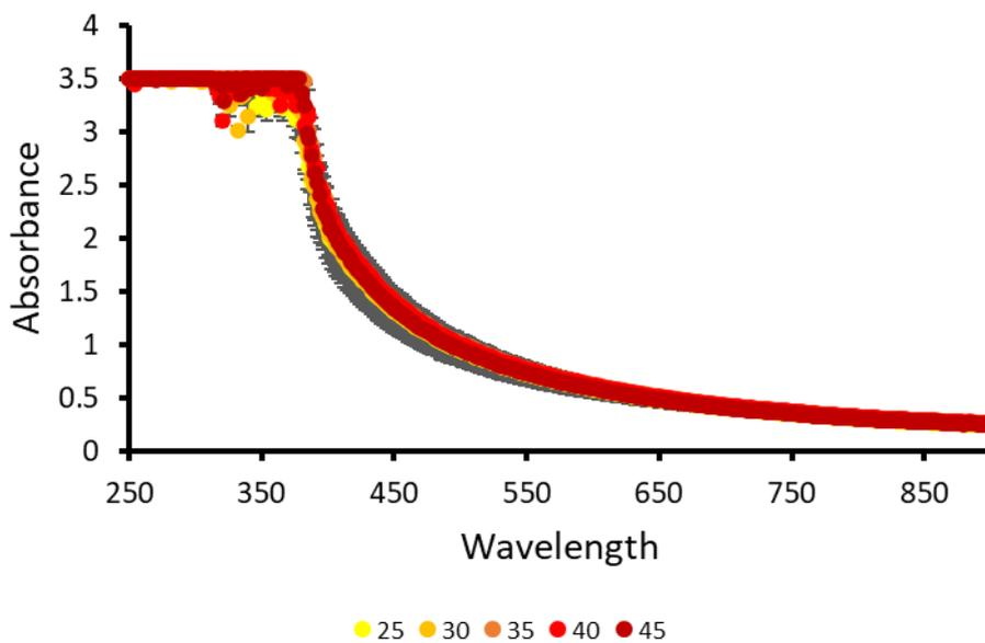
Figure S180 - Average (n=3) absorbance graph of **7** (1.5 mg/mL) in KCl recorded for each 200  $\mu$ L sample at 5-degree increments from 25-45  $^{\circ}$ C. Error = standard deviation of the mean.
