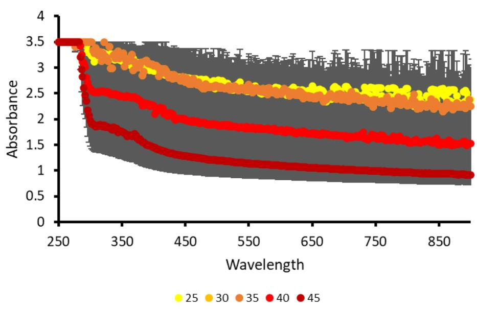
Figure S174 - Average (n=3) absorbance graph of **6** (1.5 mg/mL) in NaH<sub>2</sub>PO<sub>4</sub> recorded for each 200  $\mu$ L sample at 5-degree increments from 25-45 °C. Error = standard deviation of the mean.
