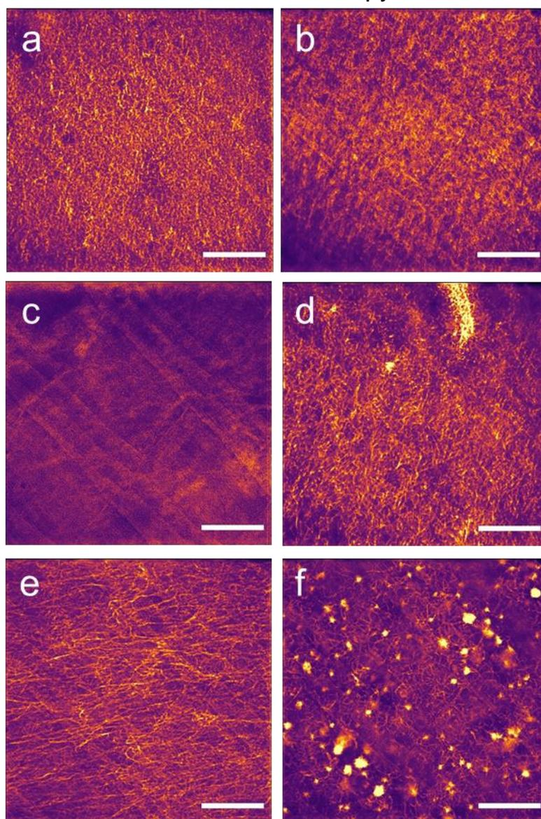
Figure S106 - Fluorescent microscopy image of **2** (5 mg/mL) in a) NaCl, b) KCl, c) NaNO<sub>3</sub>, d) NaH<sub>2</sub>PO<sub>4</sub>, e) NaOBz, f) Na<sub>2</sub>SO<sub>4</sub> at 0.505 M. Scale bar = 120 μm.
