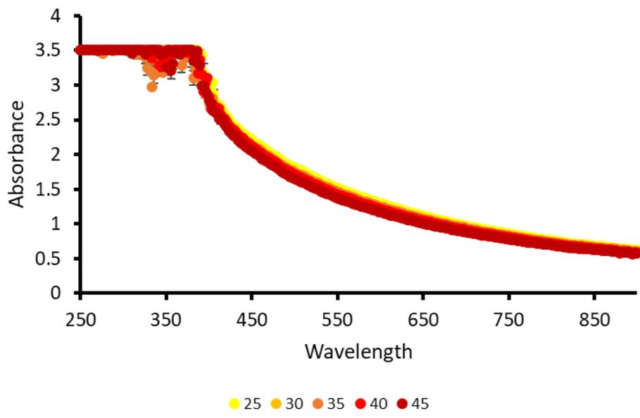
Figure S171 - Average (n=3) absorbance graph of **6** (1.5 mg/mL) in NaCl recorded for each 200  $\mu$ L sample at 5-degree increments from 25-45  $^{\circ}$ C. Error = standard deviation of the mean.
