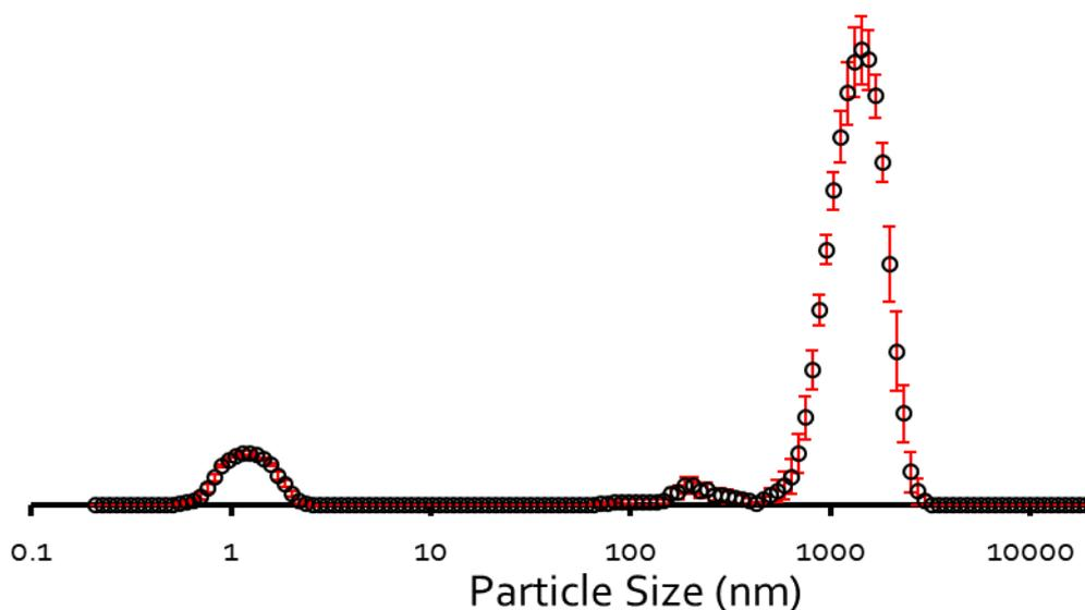
Figure S59 - The average intensity particle size distribution calculated (1380 nm) using 10 DLS runs for SSA 7 (111.2 mM) in a DMSO solution at 298 K. These data should be treated with caution due high levels of polydispersity and amorphous nature of those aggregated species produced, as indicated by quality of the data collected.
