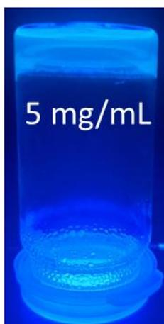
Figure S81 – SSA 3 MGC determination in 0.505 M aqueous KCl. Liquid could be seen seeping out of the material and the meniscus could be seen. MGC is above 5 mg/mL.
