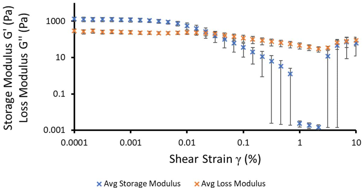
Figure S100 - Graph showing average results (n=3) from amplitude sweep experiments used to define the linear viscoelastic region of the sample at 298 K. SSA 7 (5 mg) in 1 mL of aqueous  $\text{NaNO}_3$  solution (0.505 M) (10 = 1000 %). Error = standard deviation of the mean.
