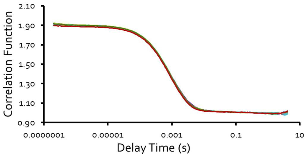
Figure S54 – Correlation function data for 10 DLS runs of SSA 7 (5.56 mM) in an EtOH: H<sub>2</sub>O (1:19) solution at 298K.
