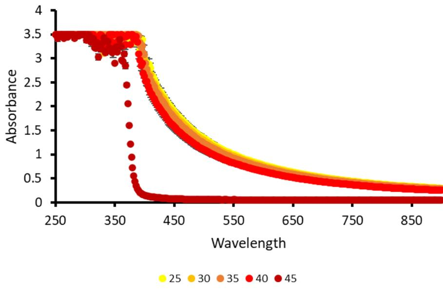
Figure S181 - Average (n=3) absorbance graph of 7 (1.5 mg/mL) in NaNO<sub>3</sub> recorded for each 200 μL sample at 5-degree increments from 25-45 °C. Error = standard deviation of the mean.
