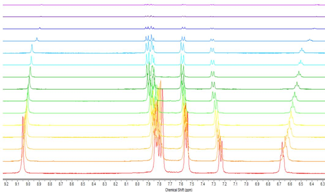
Figure S27 - Enlarged  $^1\text{H}$  NMR stack plot of SSA **4** in a  $\text{DMSO-}d_6$  0.5 %  $\text{H}_2\text{O}$  solution. Samples were prepared in series with an aliquot of the most concentrated solution undergoing serial dilution.
