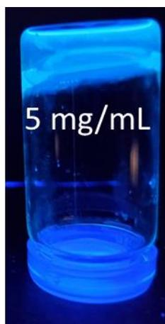
Figure S89 – SSA 4 MGC determination in 0.505 M aqueous  $\text{NaH}_2\text{PO}_4$ . Liquid could be seen seeping out of the material and the meniscus could be seen. MGC is above 5 mg/mL.
