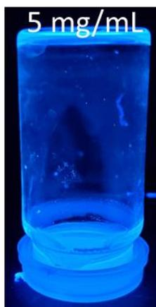
Figure S97 – SSA 7 MGC determination in 0.505 M aqueous  $\text{Na}_2\text{SO}_4$ . Hydrogel not formed at 5 mg/mL.
