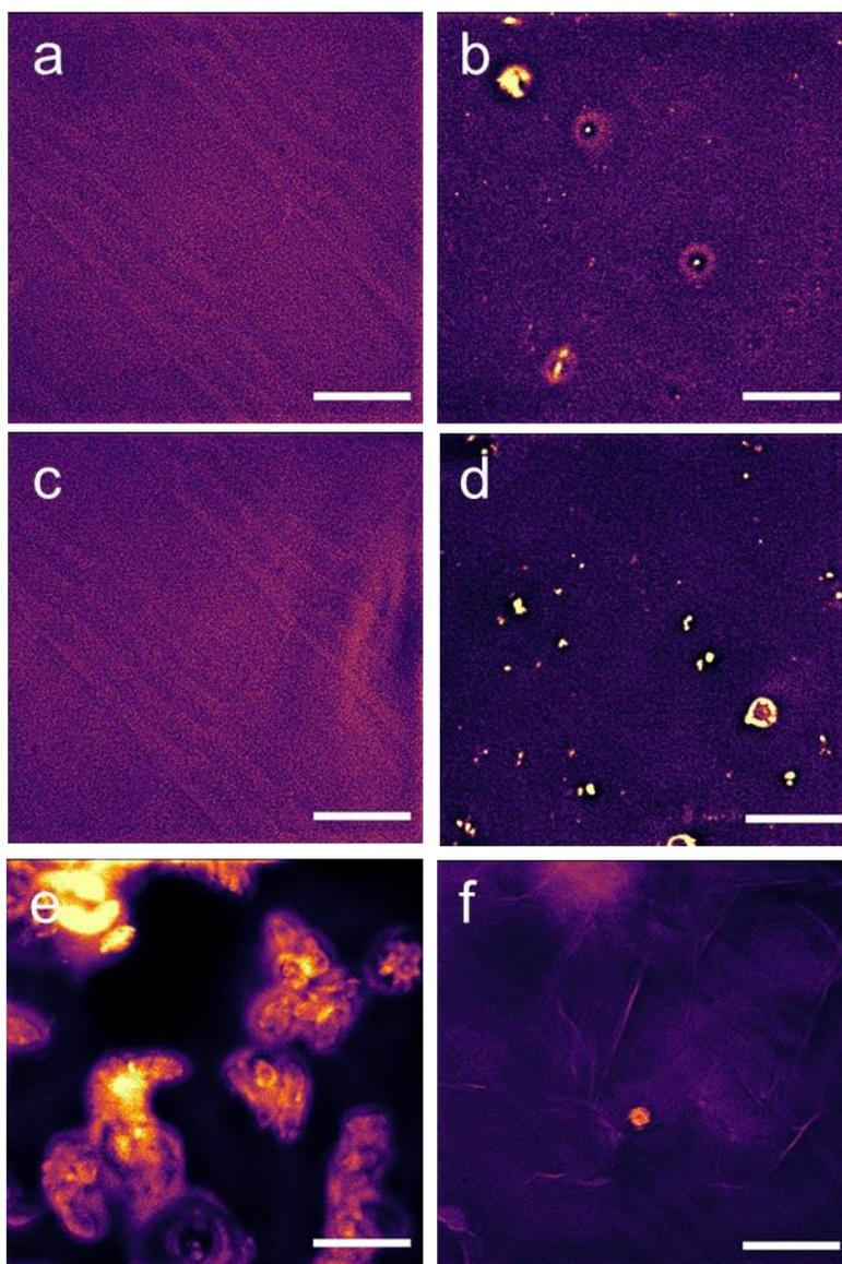
Figure S109 - Fluorescent microscopy image of **5** (5 mg/mL) in a) NaCl, b) KCl, c) NaNO<sub>3</sub>, d) NaH<sub>2</sub>PO<sub>4</sub>, e) NaOBz, f) Na<sub>2</sub>SO<sub>4</sub> at 0.505 M. Scale bar = 120 μm.
