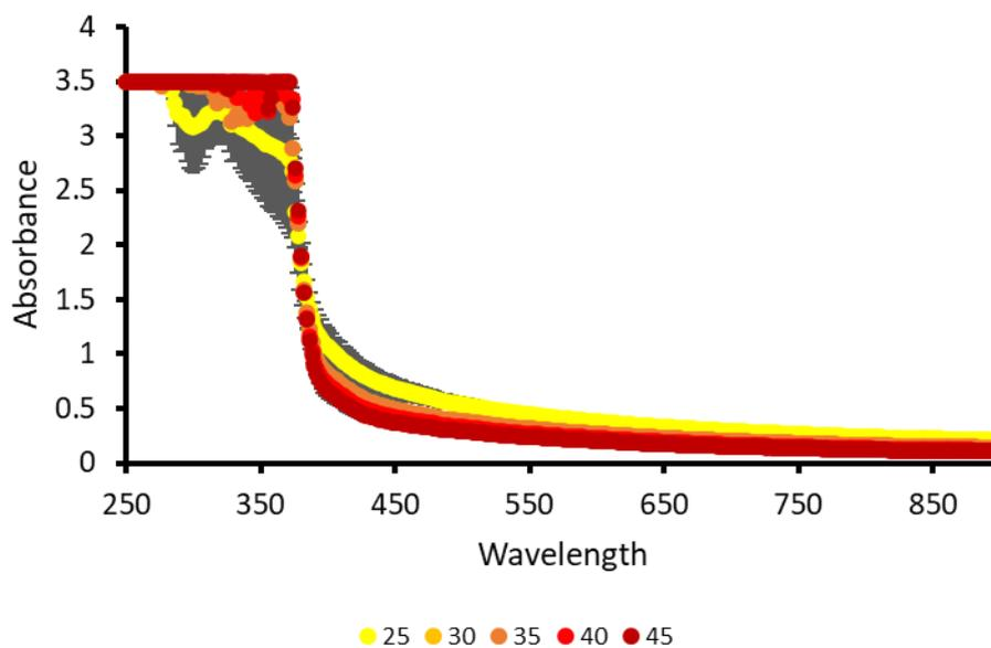
Figure S176 - Average (n=3) absorbance graph of **6** (1.5 mg/mL) in Na<sub>2</sub>SO<sub>4</sub> recorded for each 200  $\mu$ L sample at 5-degree increments from 25-45  $^{\circ}$ C. Error = standard deviation of the mean.
