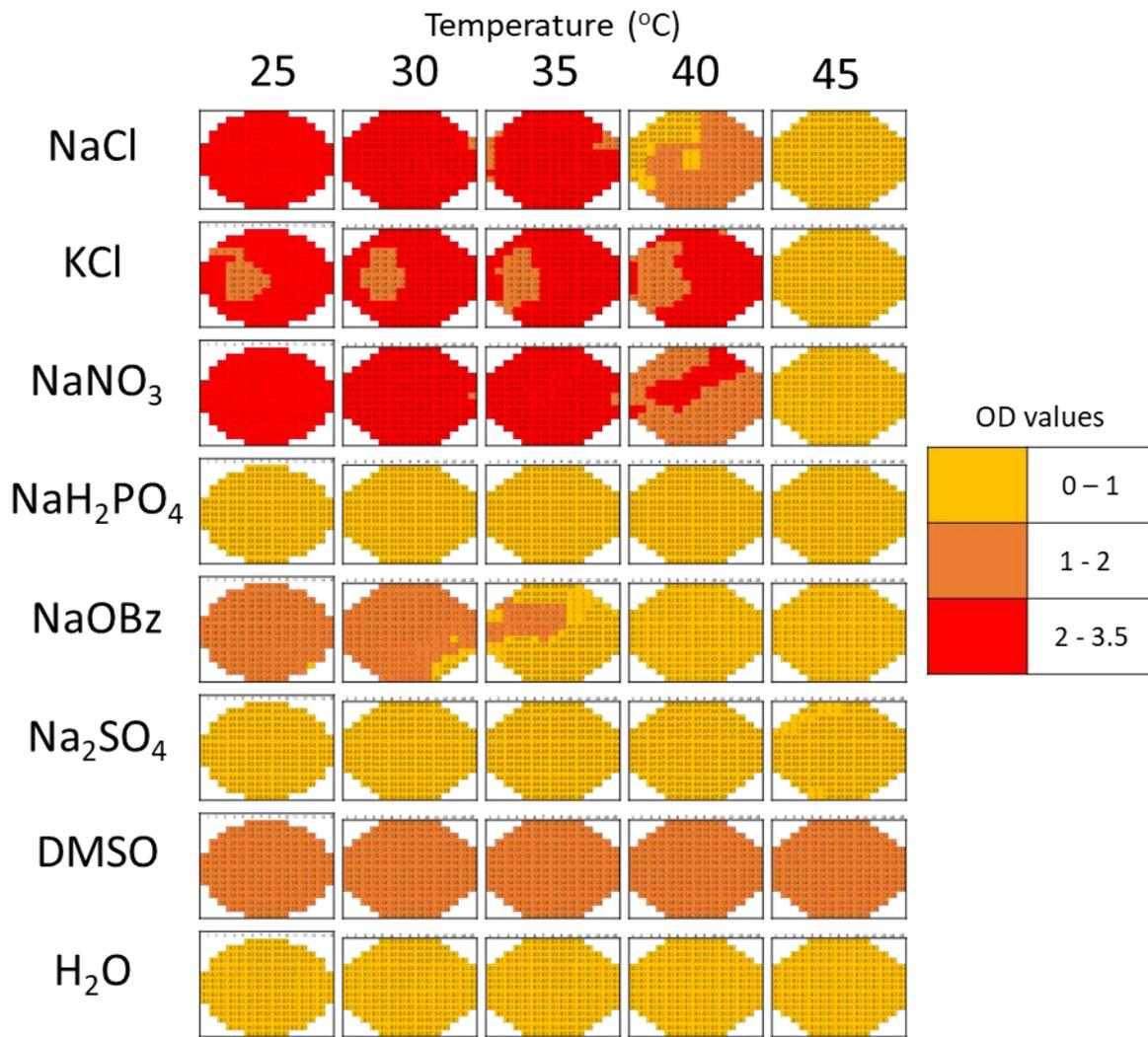
Figure S191 - Well scans (n=3) conducted at OD<sub>495</sub> at a range of temperatures for SSA 7.
