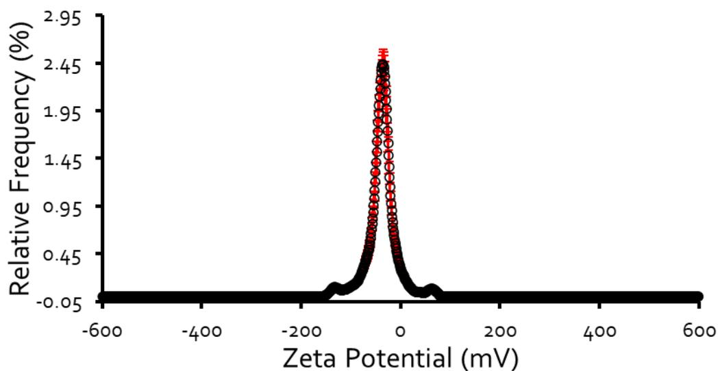
Figure S60 - The average zeta potential distribution calculated using 10 runs for SSA 1 (0.56 mM) in EtOH:H<sub>2</sub>O (1:19) solution at 298 K. Average measurement value -42.71 mV.
