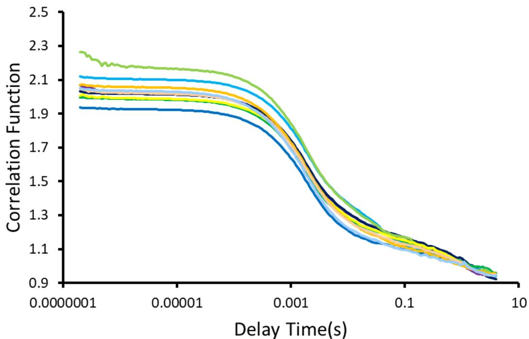
Figure S52 - Correlation function data for 10 DLS runs of SSA **6** (0.28 mM) in an EtOH:H<sub>2</sub>O (1:19) solution at 298 K.
