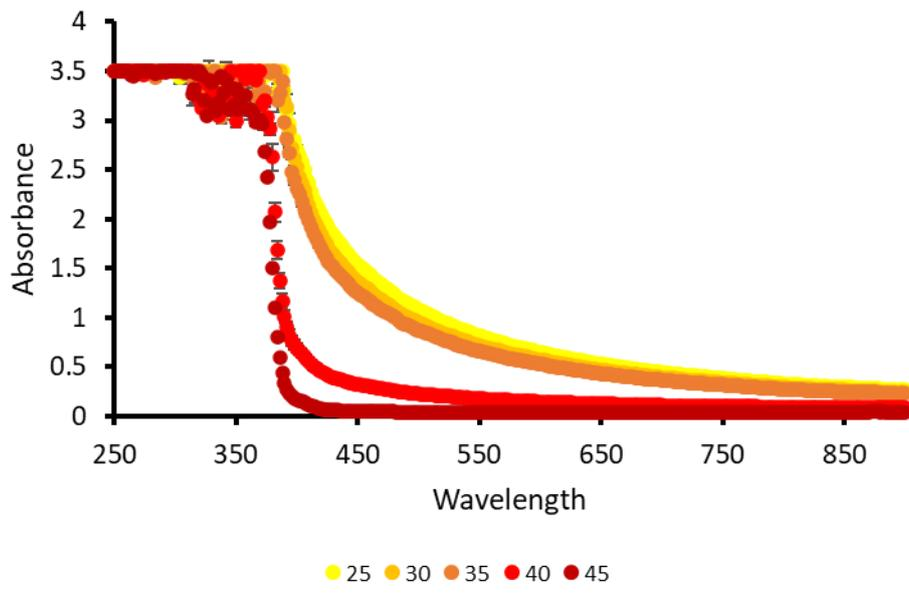
Figure S155 - Average (n=3) absorbance graph of 4 (1.5 mg/mL) in NaCl recorded for each 200  $\mu$ L sample at 5-degree increments from 25-45  $^{\circ}$ C. Error = standard deviation of the mean.
