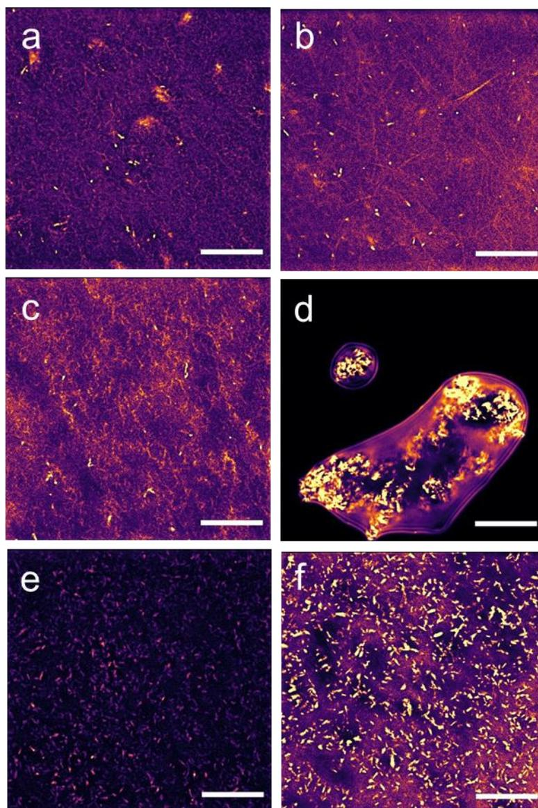
Figure S110 - Fluorescent microscopy image of **6** (5 mg/mL) in a) NaCl, b) KCl, c) NaNO<sub>3</sub>, d) NaH<sub>2</sub>PO<sub>4</sub>, e) NaOBz, f) Na<sub>2</sub>SO<sub>4</sub> at 0.505 M. Scale bar = 120 μm.
