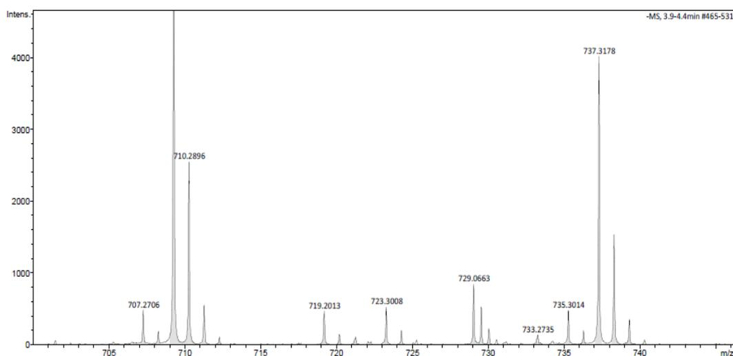
Figure S79 – A high-resolution mass spectrum (ESI<sup>-</sup>) obtained for dimeric species of SSA 7 in methanol,  $m/z$  [ $M + M + H^+$ ].
