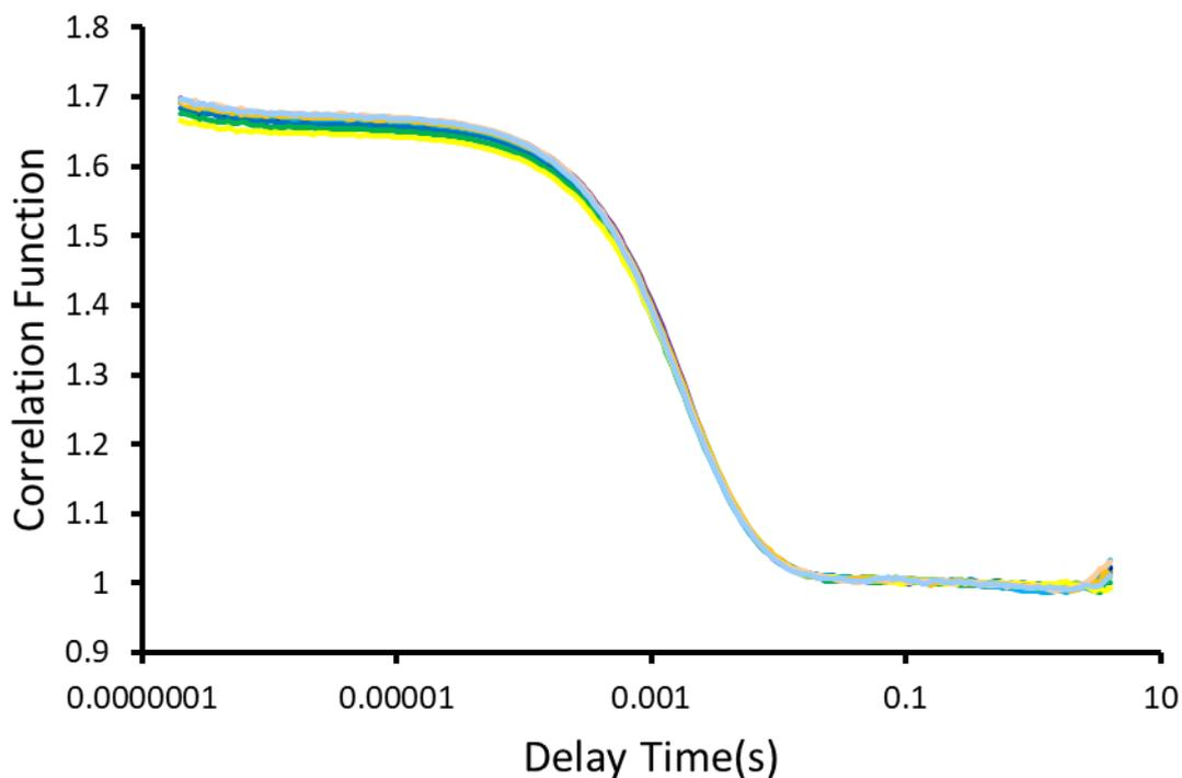
Figure S42 - Correlation function data for 10 DLS runs of SSA **3** (5.56 mM) in an EtOH:H<sub>2</sub>O (1:19) solution at 298 K.
