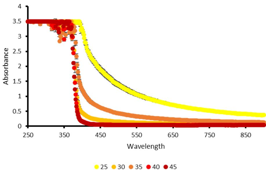
Figure S160 - Average (n=3) absorbance graph of **4** (1.5 mg/mL) in Na<sub>2</sub>SO<sub>4</sub> recorded for each 200  $\mu$ L sample at 5-degree increments from 25-45  $^{\circ}$ C. Error = standard deviation of the mean.
