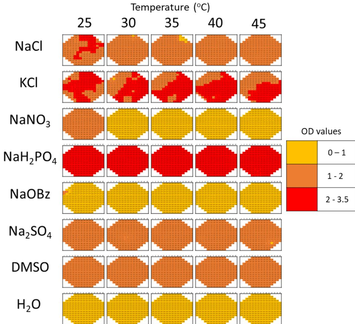
Figure S189 - Well scans (n=3) conducted at OD<sub>495</sub> at a range of temperatures for SSA 5.
