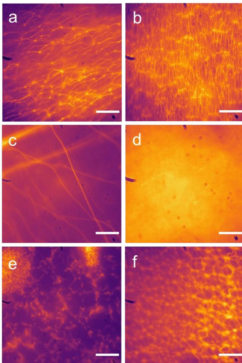
Figure S107 - Fluorescent microscopy image of **3** (5 mg/mL) in a) NaCl, b) KCl, c) NaNO<sub>3</sub>, d) NaH<sub>2</sub>PO<sub>4</sub>, e) NaOBz, f) Na<sub>2</sub>SO<sub>4</sub> at 0.505 M. Scale bar = 20 μm.
