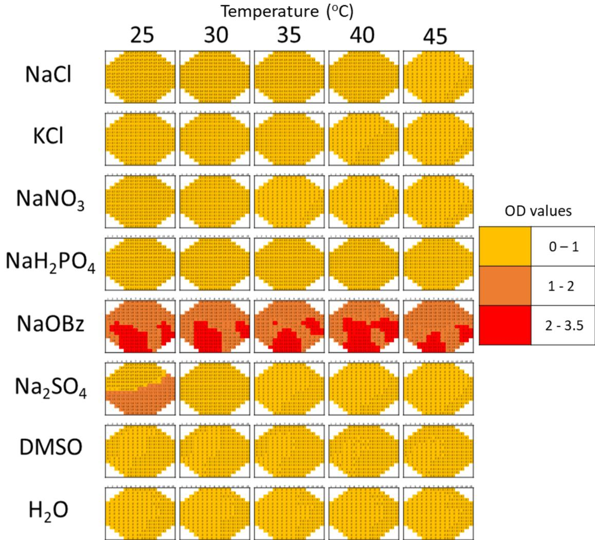
Figure S188 - Well scans (n=3) conducted at OD<sub>495</sub> at a range of temperatures for SSA 4.
