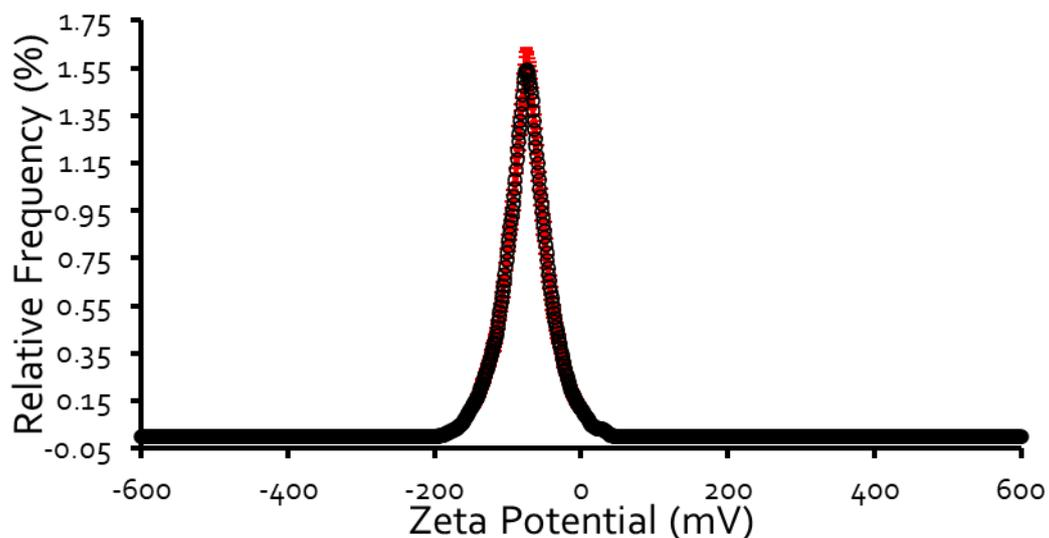
Figure S64 - The average zeta potential distribution calculated using 10 runs for SSA 7 (5.56 mM) in EtOH:H<sub>2</sub>O (1:19) solution at 298 K. Average measurement value -67.13 mV.
