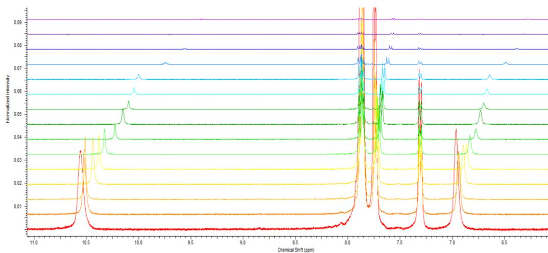
Figure S30 - Enlarged  $^1\text{H}$  NMR stack plot of SSA **6** in a  $\text{DMSO-}d_6$  0.5 %  $\text{H}_2\text{O}$  solution. Samples were prepared in series with an aliquot of the most concentrated solution undergoing serial dilution.
