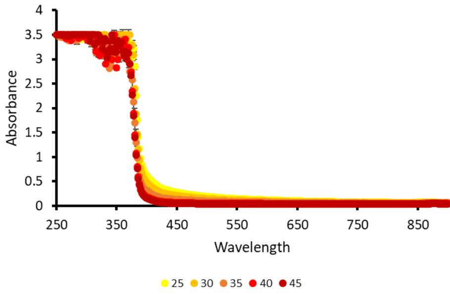
Figure S156 - Average (n=3) absorbance graph of 4 (1.5 mg/mL) in KCl recorded for each 200  $\mu$ L sample at 5-degree increments from 25-45  $^{\circ}$ C. Error = standard deviation of the mean.
