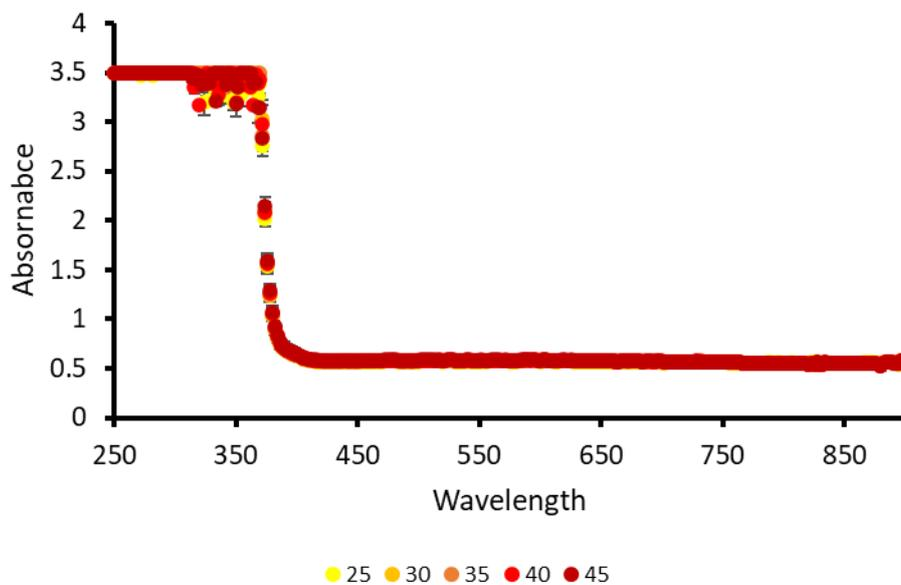
Figure S153 - Average (n=3) absorbance graph of **3** (1.5 mg/mL) in DMSO recorded for each 200  $\mu$ L sample at 5-degree increments from 25-45  $^{\circ}$ C. Error = standard deviation of the mean.
