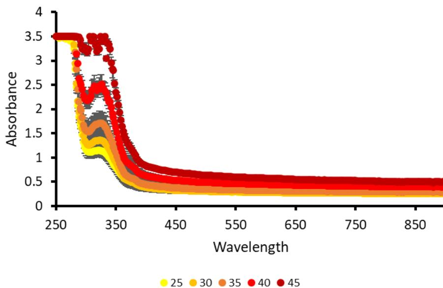
Figure S184 - Average (n=3) absorbance graph of **7** (1.5 mg/mL) in Na<sub>2</sub>SO<sub>4</sub> recorded for each 200  $\mu$ L sample at 5-degree increments from 25-45  $^{\circ}$ C. Error = standard deviation of the mean.
