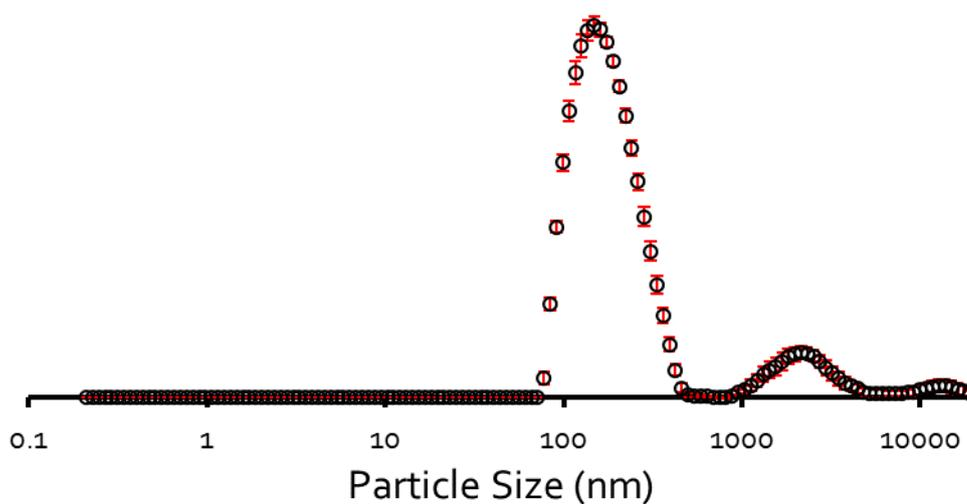
Figure S41 - The average intensity particle size distribution calculated (127 nm) using 10 DLS runs for SSA 1 (0.56 mM) in an EtOH:H<sub>2</sub>O (1:19) solution at 298 K.
