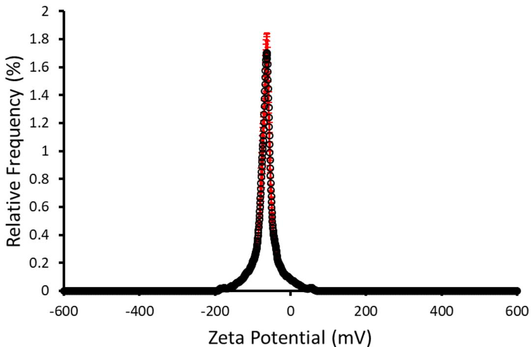
Figure S62 - The average zeta potential distribution calculated using 10 runs for SSA 4 (5.56 mM) in EtOH:H<sub>2</sub>O (1:19) solution at 298 K. Average measurement value -74.80 mV.
