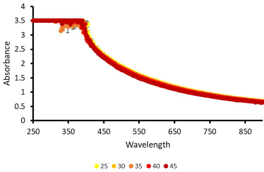
Figure S173 - Average (n=3) absorbance graph of **6** (1.5 mg/mL) in NaNO<sub>3</sub> recorded for each 200  $\mu$ L sample at 5-degree increments from 25-45 °C. Error = standard deviation of the mean.
