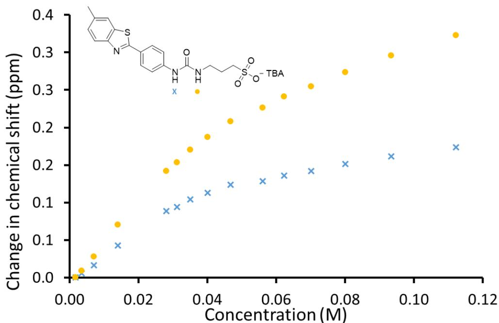
Figure S28 - Graph illustrating the  $^1\text{H}$  NMR down-field change in chemical shift of urea NH resonances with increasing concentrations of SSA 4 in  $\text{DMSO-}d_6$  0.5 %  $\text{H}_2\text{O}$  solution (298 K).
