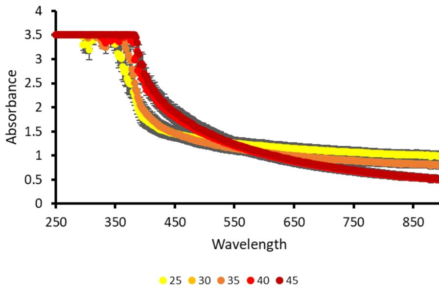
Figure S175 - Average (n=3) absorbance graph of **6** (1.5 mg/mL) in NaOBz recorded for each 200  $\mu$ L sample at 5-degree increments from 25-45  $^{\circ}$ C. Error = standard deviation of the mean.
