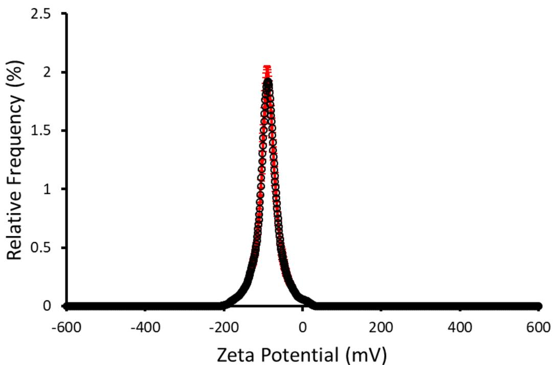
Figure S63 - The average zeta potential distribution calculated using 10 runs for SSA 6 (2.78 mM) in EtOH:H<sub>2</sub>O (1:19) solution at 298 K. Average measurement value -84.22 mV.
