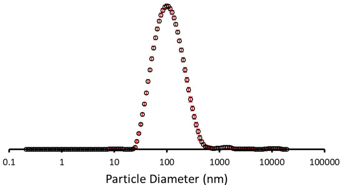
Figure S49 - The average intensity particle size distribution calculated (1320 nm) using 10 DLS runs for SSA 4 (0.56 mM) in an EtOH:H<sub>2</sub>O (1:19) solution at 298 K.
