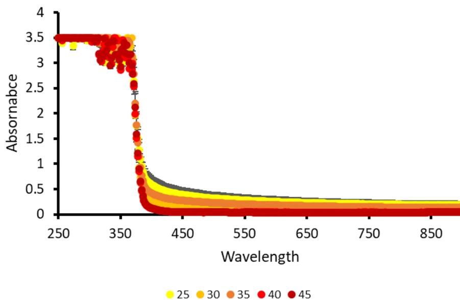
Figure S152 - Average (n=3) absorbance graph of **3** (1.5 mg/mL) in Na<sub>2</sub>SO<sub>4</sub> recorded for each 200  $\mu$ L sample at 5-degree increments from 25-45 °C. Error = standard deviation of the mean.
