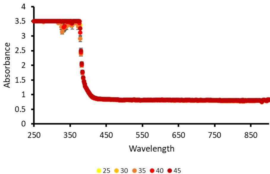
Figure S177 - Average (n=3) absorbance graph of **6** (1.5 mg/mL) in DMSO recorded for each 200  $\mu$ L sample at 5-degree increments from 25-45  $^{\circ}$ C. Error = standard deviation of the mean.
