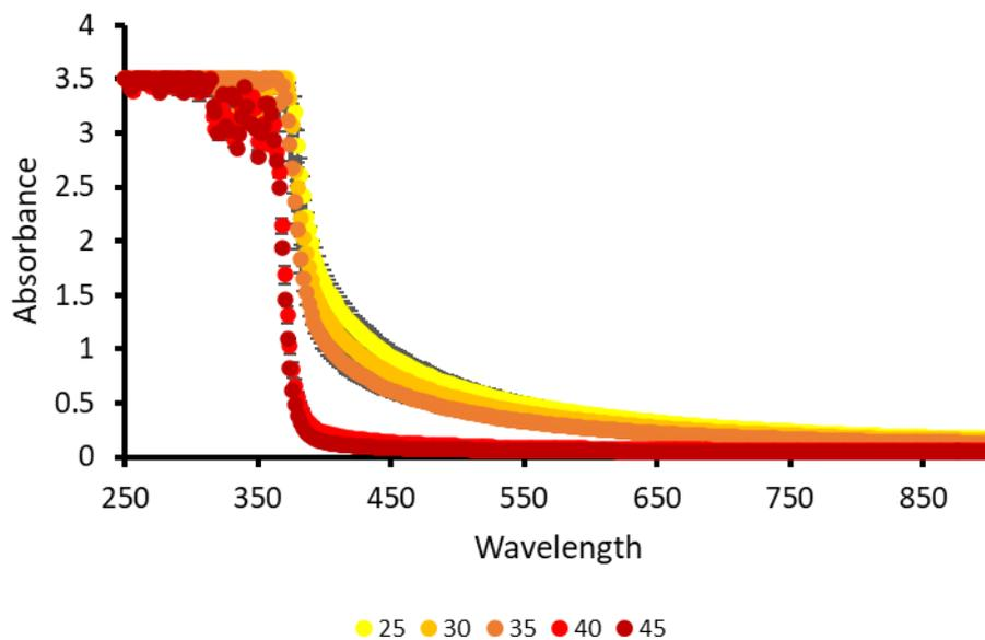
Figure S183 - Average (n=3) absorbance graph of **7** (1.5 mg/mL) in NaOBz recorded for each 200  $\mu$ L sample at 5-degree increments from 25-45  $^{\circ}$ C. Error = standard deviation of the mean.
