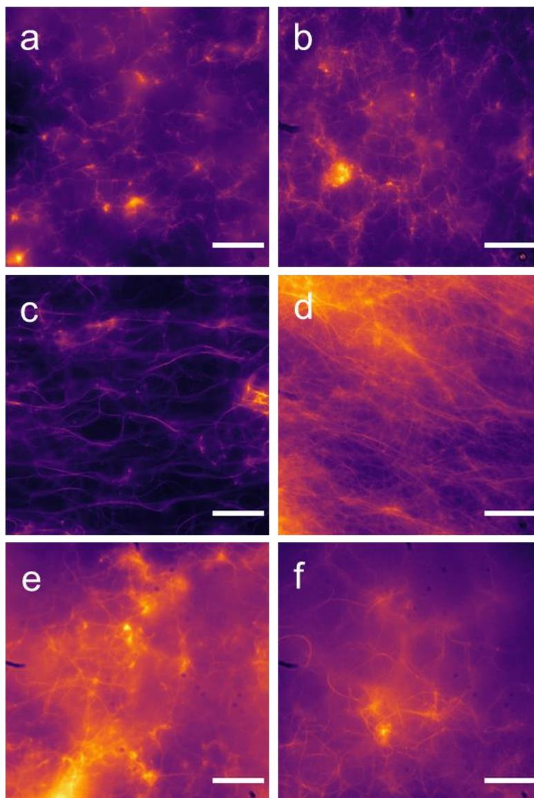
Figure S111 - Fluorescent microscopy image of **7** (5 mg/mL) in a) NaCl, b) KCl, c) NaNO<sub>3</sub>, d) NaH<sub>2</sub>PO<sub>4</sub>, e) NaOBz, f) Na<sub>2</sub>SO<sub>4</sub> at 0.505 M. Scale bar = 20 μm.
