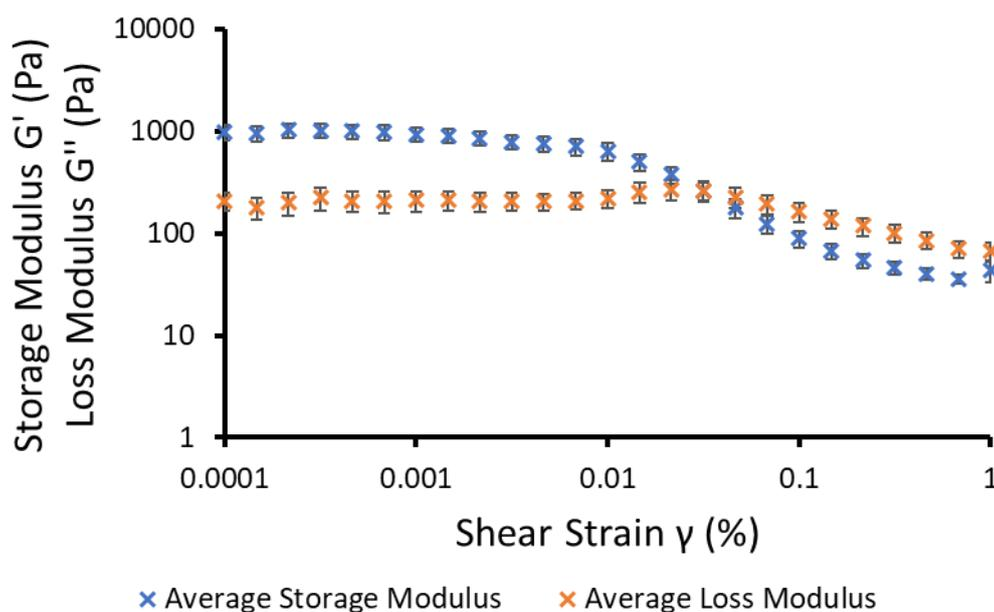
Figure S98 - Graph showing average results ( $n=3$ ) from amplitude sweep experiments used to define the linear viscoelastic region of the sample at 298 K. SSA 7 (5 mg) in 1 mL of aqueous NaCl solution (0.505 M) (1 = 100 %). Error = standard deviation of the mean.
