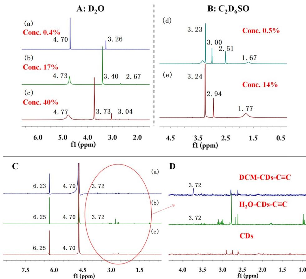
**Figure S2.**  $^1\text{H}$  NMR spectra of mono-propargylamine in (A)  $\text{D}_2\text{O}$  and (B)  $\text{C}_2\text{D}_6\text{SO}$  with different concentrations; (C)  $^1\text{H}$  NMR spectra of (a) DCM-CDs-C $\equiv$ C, (b) H $_2$ O-CDs-C $\equiv$ C, and (c) CDs; (D) a partial enlargement of Figure C.
