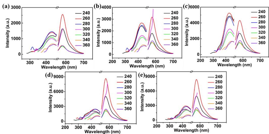
**Figure S5.** PL spectra of CDs-RhB with different ratios of RhB-N<sub>3</sub>' mole to CDs-C≡C' mass: (a) 0.52, (b) 0.76, (c) 1.54, (d) 3.08, and (e) 4.16,  $\times 10^{-3}$  mmol/mg, ex- and em- slit: 10 nm.
