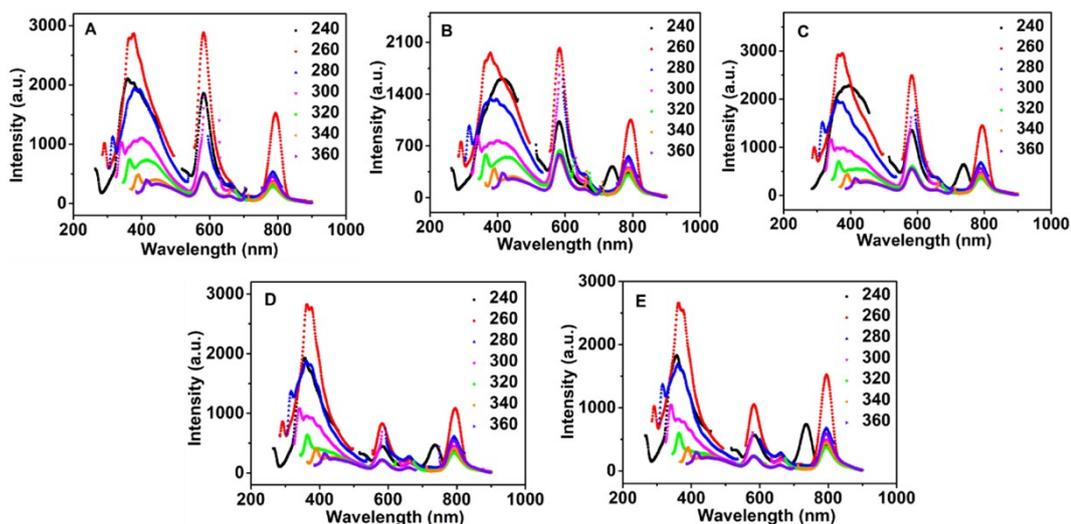
**Figure S7.** PL spectra of CDs-RhB/Cy7 with different molar ratios of RhB-N<sub>3</sub> to Cy7-N<sub>3</sub>: (A) 5:1, (B) 2:1, (C) 1:1, (D) 1:2, and (E) 1:5, ex- and em- slit: 10 nm.
