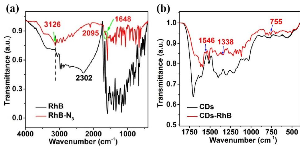
**Figure S1.** FTIR spectra of (a) RhB and RhB-N<sub>3</sub>; (b) CDs and CDs-RhB.
