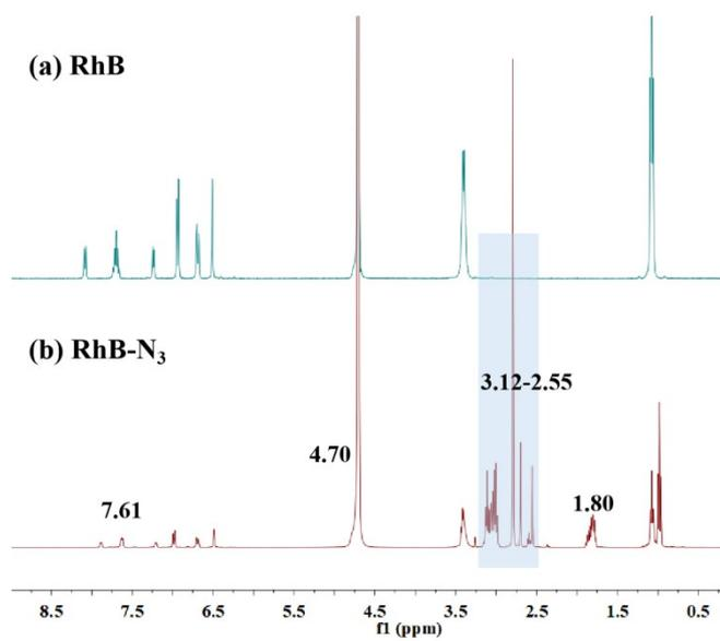
**Figure S4.** <sup>1</sup>H NMR spectra of (a) RhB and (b) RhB-N<sub>3</sub> in D<sub>2</sub>O.
