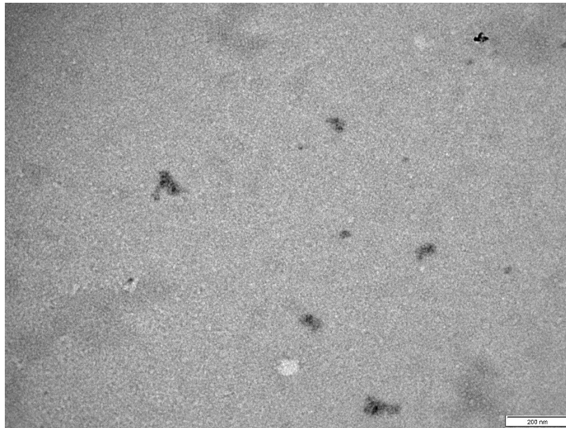
Figure S1 – Characterization of ssDNA micelles using TEM imaging, showing the poorly formed micellar structures with uneven shape and size.
