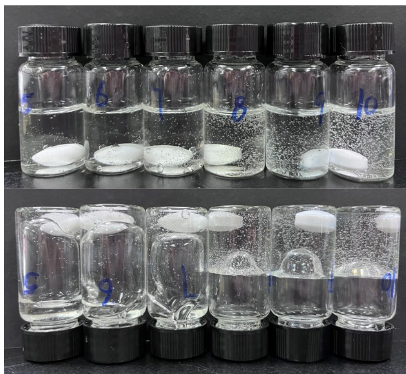
Fig. S2. Mobility comparison of different concentrations of HA (from left to right, the concentrations of HA are 5%-10% respectively).
