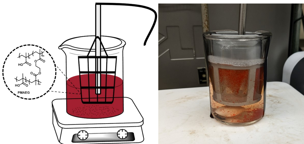
Figure S1. Illustration of DOX capture set-up using UV probe and filter. The polymer composites were stirred continually in DOX–PBS solution beneath the filter.
