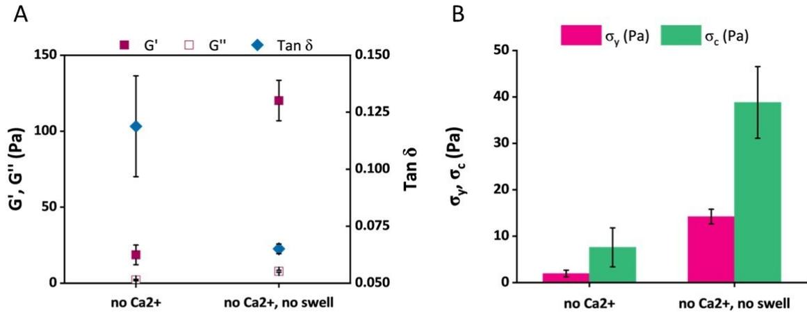
**Figure S5.** Effect of Ca<sup>2+</sup> ions on rheological properties of the hydrogel films. (A) Rest and (B) yield properties of 0.05 wt% LVMLG-TCNF matrices without Ca<sup>2+</sup>-ions. One set of samples was prepared as the MLG-Ca<sup>2+</sup>-TCNF matrices in water, and the other in a similar manner without letting the gel films swell overnight prior to the rheological measurements.
