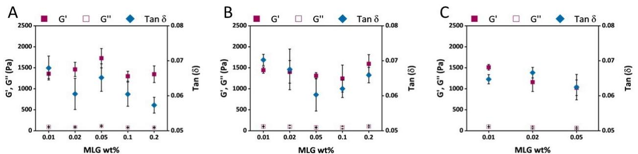
**Figure S4.** Rest properties of self-standing hydrogel films.  $G'$ ,  $G''$ , and  $\tan \delta$  of (A) LVMLG- $\text{Ca}^{2+}$ -TCNF, (B) MVMLG- $\text{Ca}^{2+}$ -TCNF, and (C) HVMLG- $\text{Ca}^{2+}$ -TCNF matrices with varying cross-linker concentration in LVE region at 1 Pa. Standard deviations are shown.
