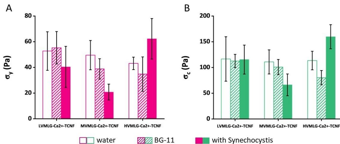
**Figure 56.** Comparison of yielding behaviour of MLG-Ca<sup>2+</sup>-TCNF matrices. (A)  $\sigma_y$  and (B)  $\sigma_c$  of the self-standing hydrogel films prepared in water, BG-11 growth medium without cells, and in suspension of Synechocystis cells. Cross-linker concentration of 0.01 wt% was used for HV- and MVMLG-Ca<sup>2+</sup>-TCNF matrices, and 0.05 wt% for LVMLG-Ca<sup>2+</sup>-TCNF. Standard deviations are shown.
