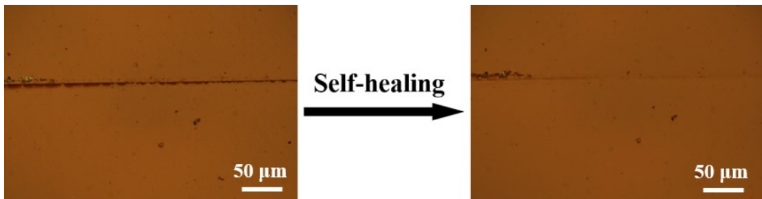
Fig. S12 The optical microscope photographs of MPI-2 after scratching and self-healing.
