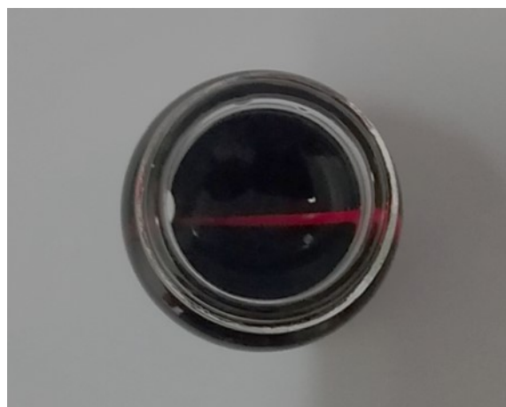
Fig. S1. Digital image of MXene aqueous solution with a typical Tyndall effect.
