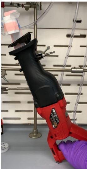
SI Figure 1. Image of custom emulsion mixer used to mix the aqueous phase into the organic phase of the emulsion.
