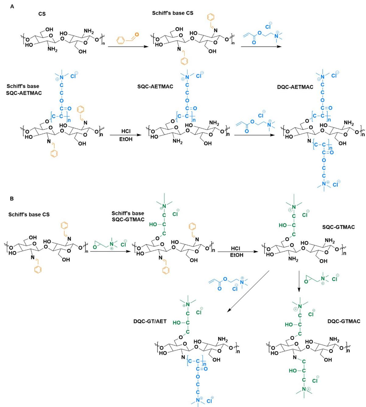
**Scheme S1.** Reaction schemes of the preparation of quaternized chitosan with **(A)** AETMAC and **(B)** GTMAC.
