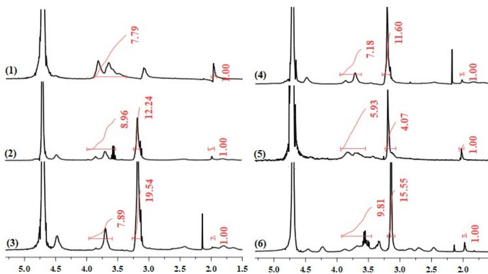
**Figure S2.**  $^1\text{H-NMR}$  spectra and integrals used for the determination of the degree of quaternization (dQ) and deacetylation (DDA), where 1-6 is chitosan, SQC-AETMAC, DQC-AETMAC, DQC-GT/AET, SQC-GTMAC, and DQC-GTMAC.
