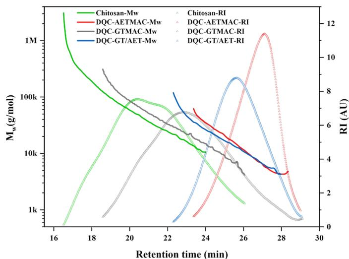
**Figure S4.** Results of GPC analysis: the obtained molecular weight ( $M_w$ ) and refractive index (RI) versus their respective elution time of chitosan and DQCs.
