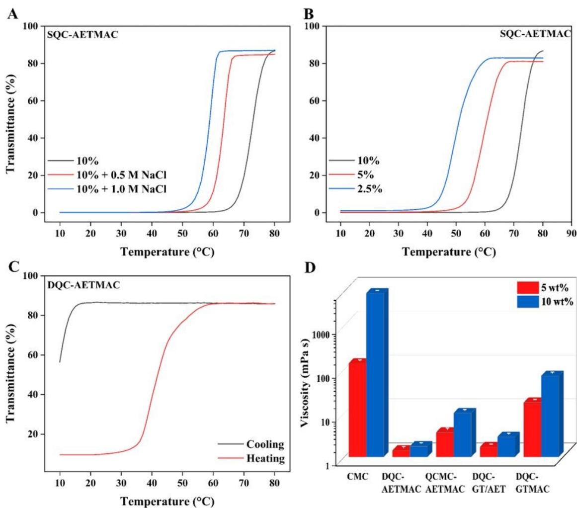
**Figure S6.** (A, B) UCST behavior of SQC-AETMAC during heating 10-80 °C, at different concentrations and with the addition of NaCl. (C) UCST behavior of DQC-AETMAC at a concentration of 10 % (w/v). (D) viscosity ( $\log_{10}$ ) of CMC and DQCs at 5 and 10 % (w/v) concentrations. Chitosan and QCMC-GTMAC were excluded due to too high viscosities.
