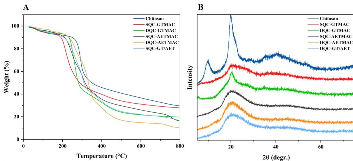
**Figure S5.** (A) TGA thermogram curves and (B) X-ray diffraction patterns of chitosan and its derivatives.
