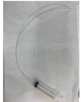
Syringe used: 10mL Capillary used: 30cm (length) et 1mm of diameter
