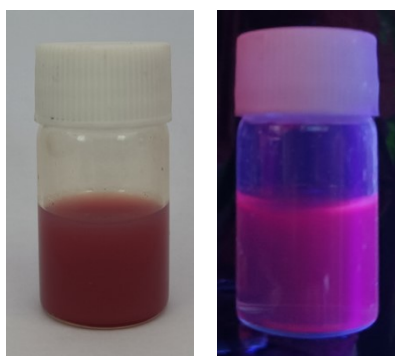
Fig. S1. HN@Cu-MOF dispersed in water under (left) ambient light and (right) UV irradiation ( \lambda = 365 nm).
