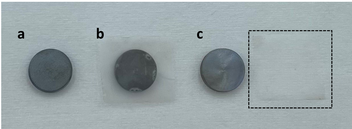
Figure S3. AgNPs adhesion test. Images showing the (a) Ag coated Ti specimen, (b) adhesive tape attachment, (c) Tape peeled off specimen with the scotch tape (dotted lines).
