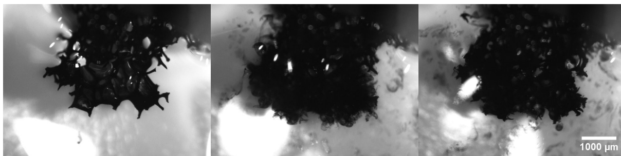
Figure S1 Representative images of a carbon sponge coated with p(g3T2) in KCl 0.01 M during pristine, expansion and contraction (from left to right, respectively).
