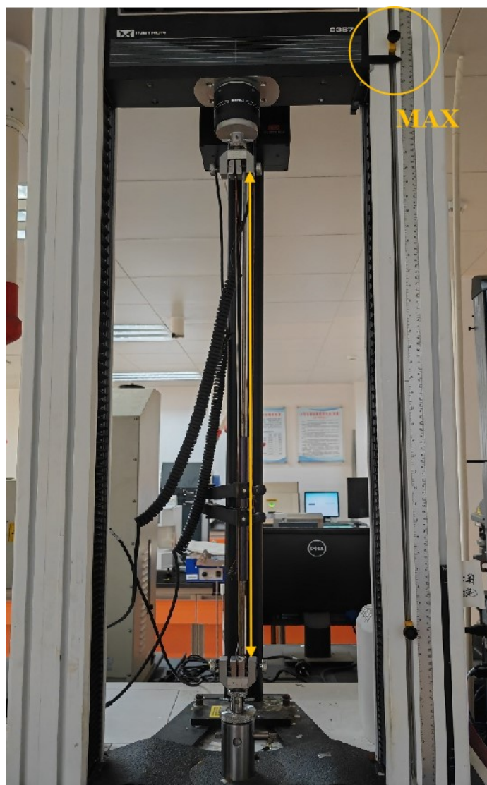
Fig. S1. The maximum elongation at break over 5500% (Strain behavior of CTPB hydrogel at the peak of test on an electronic universal testing machine)
