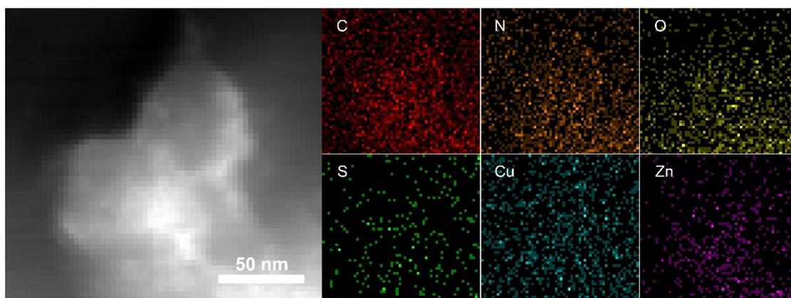
**Fig. S3** Elemental mapping images of DCZCu (scale bar = 50 nm).
