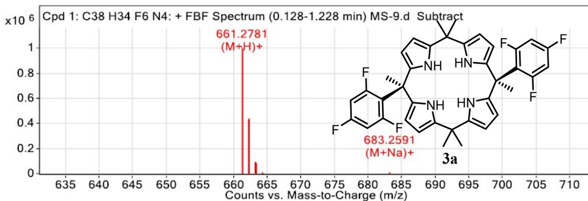
**Figure S6.** HRMS spectrum of *cis*-trifluorophenyl extended C4P (**3a**). ( $m/z$  calculated for  $\text{C}_{38}\text{H}_{34}\text{F}_6\text{N}_4$   $[\text{M}+\text{H}]^+ = 661.2760$ ).
