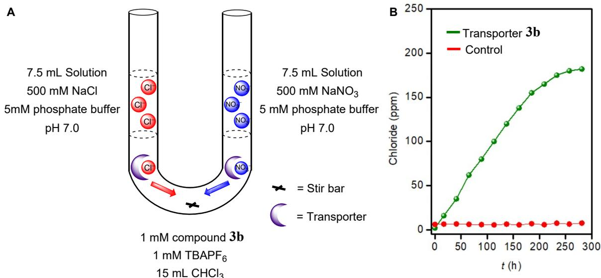
**Figure S25.** Schematic demonstration of U-tube experiment setup (A). Change of chloride ion concentration in a U-tube experiment with and without transporter **3b** (1.0 mM) (B).
