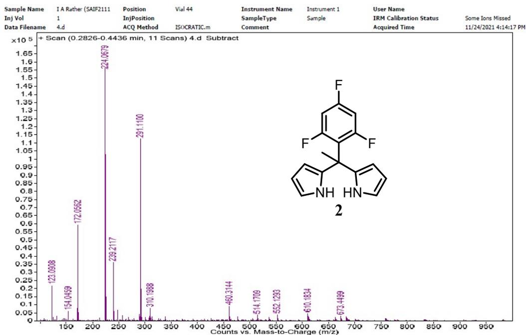
**Figure S3.** HRMS spectrum of trifluorophenyl functionalized dipyrromethane (**2**). ( $m/z$  calculated for  $C_{16}H_{13}F_3N_2 [M+H]^+ = 291.1103$ ).
