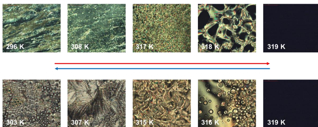
Figure S6. Polarized optical microscopy images of the heating-cooling cycles of the 8CB:azobenzene dispersion. The system behaves like pure 8CB.
