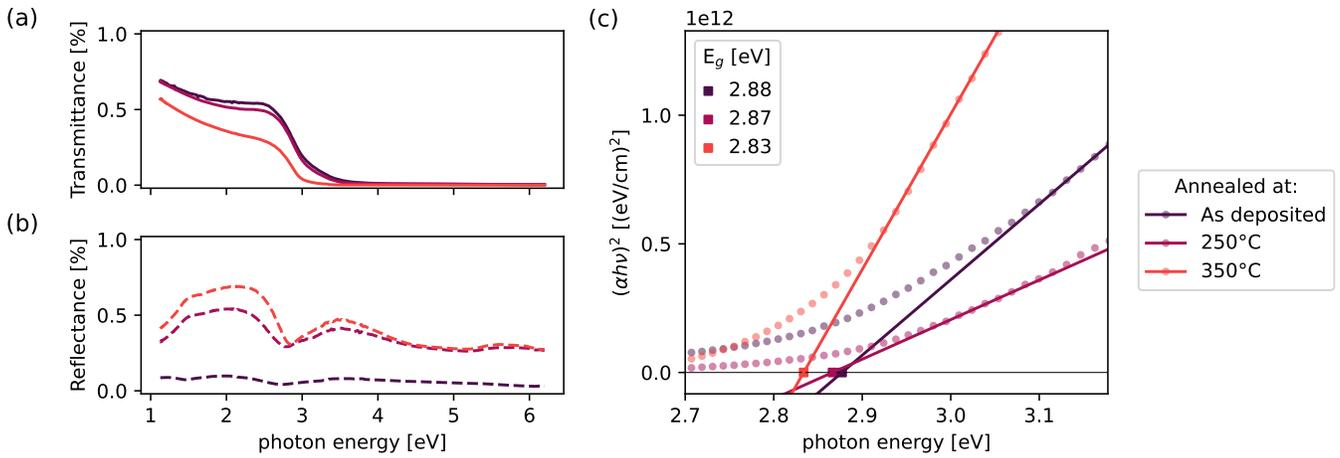
**Fig. S2** Optical properties of SnO films with varying annealing temperatures, showing: **(a)** transmittance, **(b)** reflectance and **(c)** a Tauc plot with extracted band gap energies. The films were deposited using the 3xSn with exposure mode.
