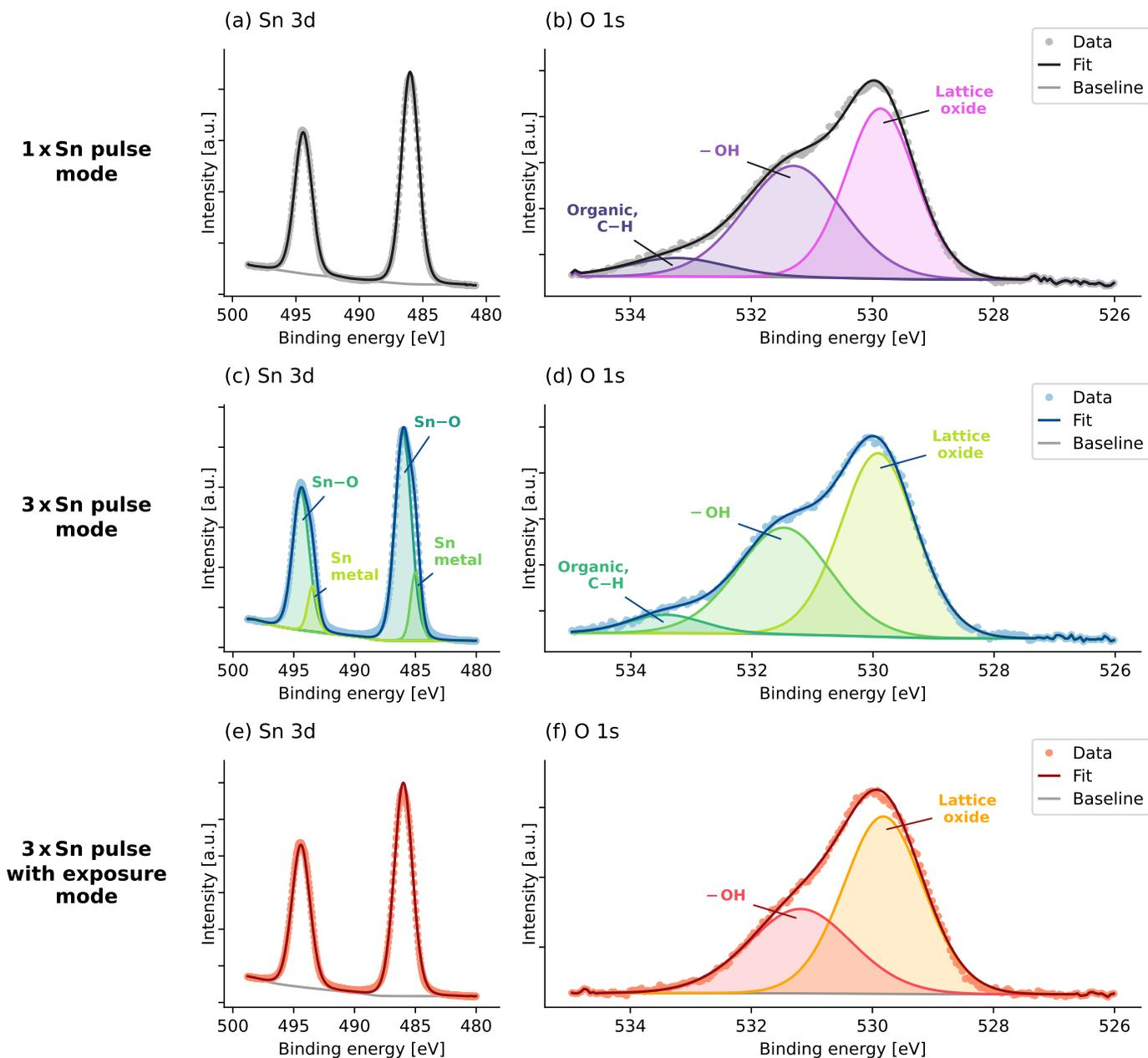
**Fig. S4** Comparison of XPS spectra of Sn 3d and O 1s core levels for the three deposition modes. XPS was performed *ex-situ*, without any etching of the SnO surface.
