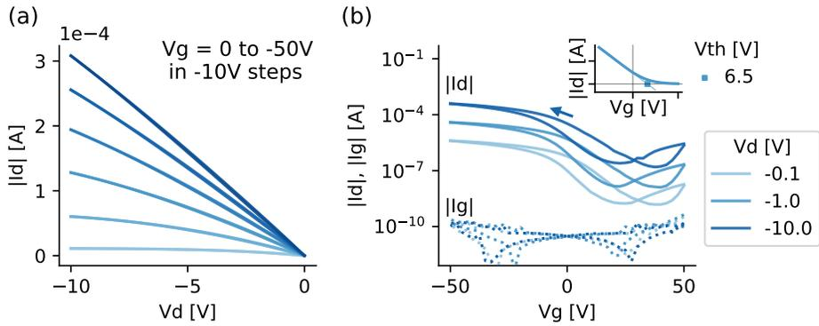
**Fig. S6** Performance of SnO TFTs deposited in 3 Sn pulse mode: **(a)** shows the output curves for  $V_g$  from 0 to -50 V; **(b)** shows the gate transfer curves ( $I_d$ ) and gate leakage current ( $I_g$ , dotted lines) for 3 values of  $V_d$ , with the extracted threshold voltage at  $V_d = -1$  V (inset).
