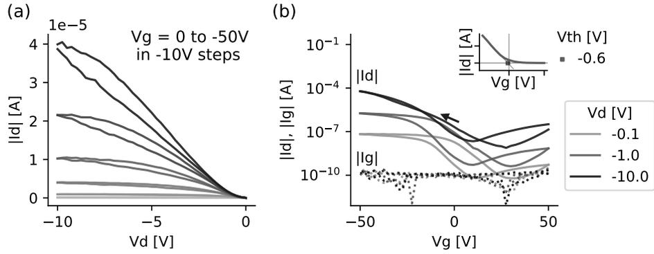
**Fig. S5** Performance of SnO TFTs deposited in single pulse mode: **(a)** shows the output curves for  $V_g$  from 0 to -50 V; **(b)** shows the gate transfer curves ( $I_d$ ) and gate leakage current ( $I_g$ , dotted lines) for 3 values of  $V_d$ , with the extracted threshold voltage at  $V_d = -1$  V (inset).
