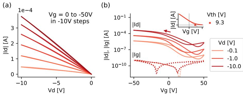
**Fig. S7** Performance of SnO TFTs deposited in 3xSn pulse with exposure mode: **(a)** shows the output curves for  $V_g$  from 0 to -50 V; **(b)** shows the gate transfer curves ( $I_d$ ) and gate leakage current ( $I_g$ , dotted lines) for 3 values of  $V_d$ , with the extracted threshold voltage at  $V_d = -1$  V (inset).
