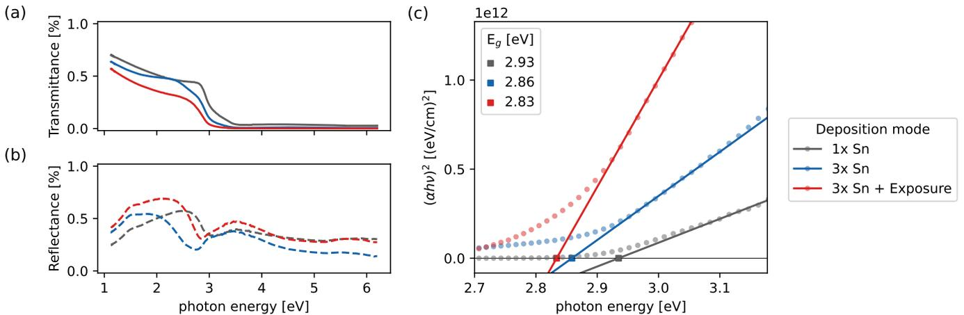
**Fig. S3** Optical properties of the SnO films for each deposition mode, showing: **(a)** transmittance, **(b)** reflectance and **(c)** a Tauc plot with extracted band gap energies. The films have all undergone post deposition annealing at 350°C.
