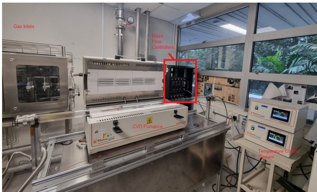
Fig. S6. CVD growth system for multilayer graphene (MLG) growth
