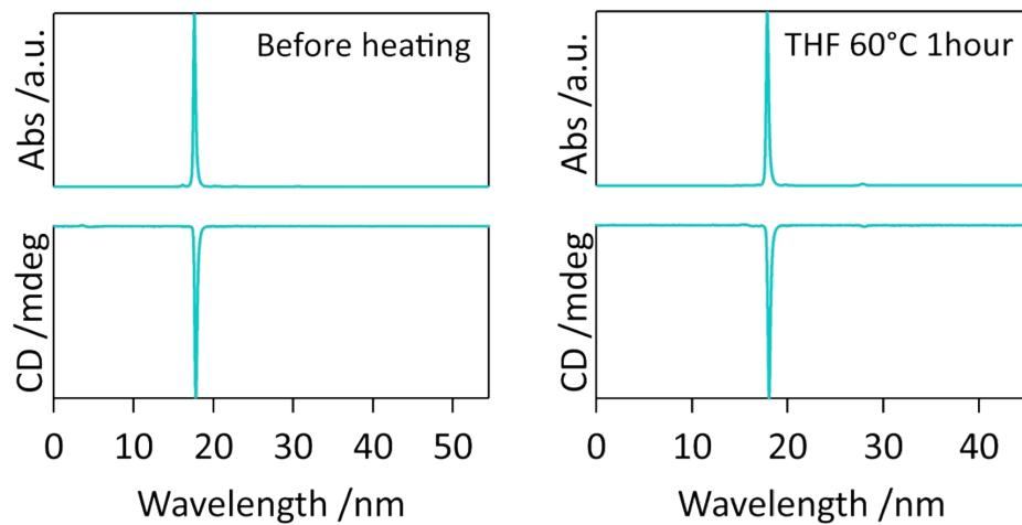
**Figure S19:** Racemization study of **DM** *S* enantiomer: the pure enantiomer was put through chiral
