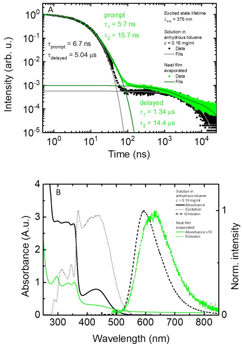
**Figure S8: A.** DM decays recorded in toluene solution (black) and in PMMA films (green) along with fitting curves and lifetimes values. **B.** DM absorption (full line), emission (dotted line) and excitation (dotted pale line) spectra in toluene (black) and in PMMA 10 wt% (green).
