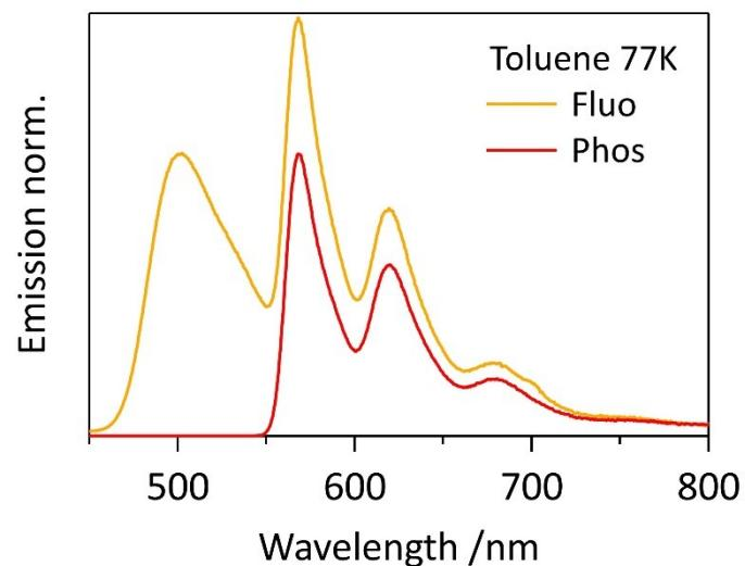
**Figure S10:** Emission spectra obtained for DM in cryostat at 77 K in toluene (C=50  $\mu$ M). Direct emission in yellow and 75 ms delayed emission in red, revealing highly structured phosphorescence emission.
