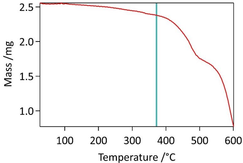
**Figure S2:** Thermogravimetric analysis of DM. The blue line indicates the point at which 5% of weight loss is observed, which happens at 372°C.
