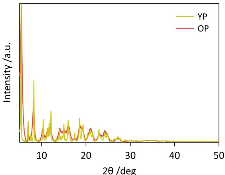
**Figure S13:** PXRD obtained from the yellow powder (**YP**) and orange powder (**OP**).
