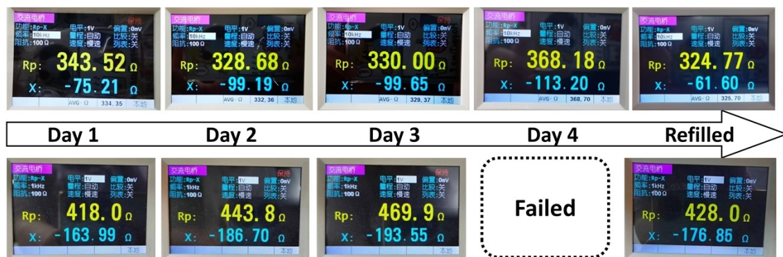
Figure S5. The image records of AC resistance within 4 days from the conductor without (upper) or with (bottom) deformation, respectively.
