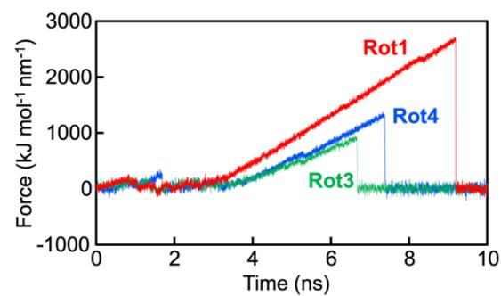
**Figure S11.** Time profiles of pulling force applied to the ring in the steered MD for **Rot1**, **Rot3**, and **Rot4** represented by red, green, and blue lines, respectively.
