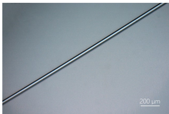
Figure S1. Optical microscope image of PbBr 2 microwire, with a diameter of 30 μm.
