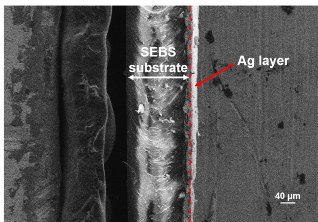
Fig. S3 The cross section of Ag/SEBS layers through screen printing.
