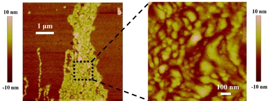
**Figure.S5** AFM image of a conductive filament. The filament area bulges significantly and is much coarser than the outside area, which indicates that the electroforming of the conductive filaments disrupts the original lattice structure.
