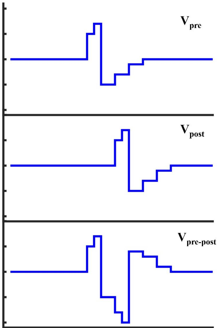
**Figure.S11** Programmed pre- and postsynaptic pulses used to emulate STDP.
