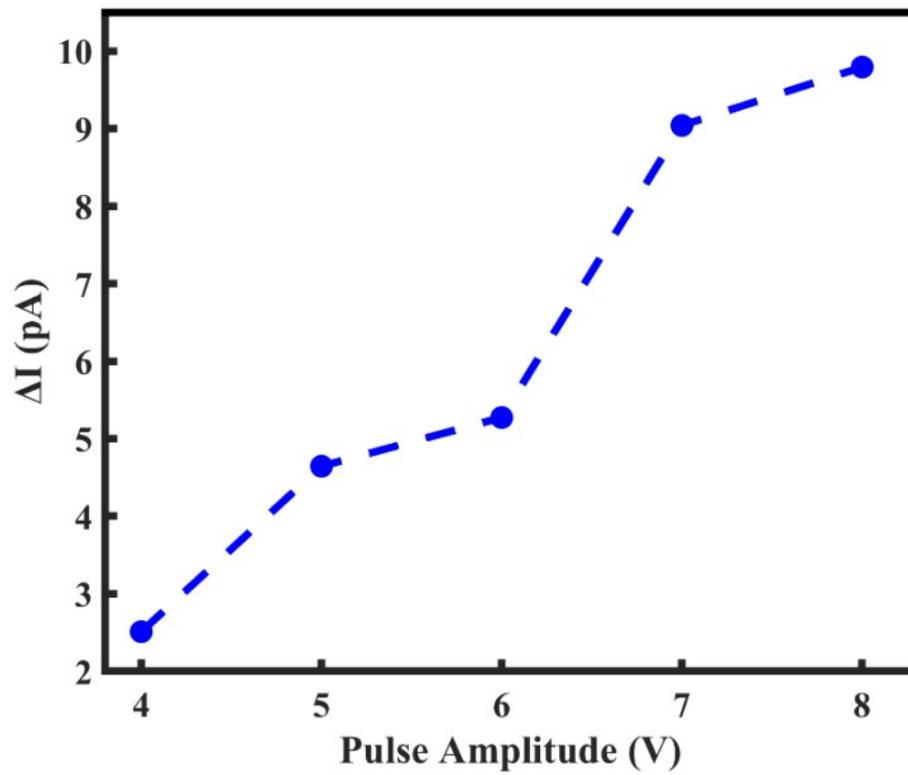
**Figure.S9** Average conductance changes caused by single pulses with different amplitudes (4 V, 5 V, 6 V, 7 V, and 8 V).
