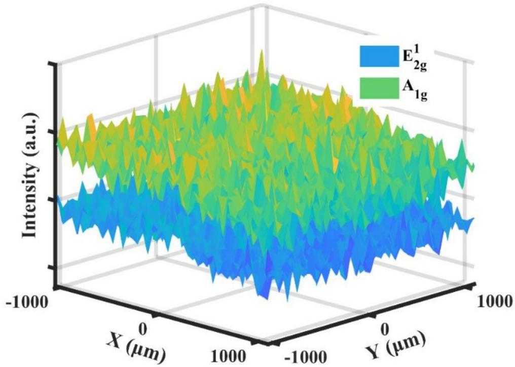
**Figure.S1** Raman mapping of MoS<sub>2</sub> film. The mapping area is 2 mm × 2 mm, and each pixel is 50 μm × 50 μm in size. The standard deviations of the peak intensities of the mapping area are 9.8% (E<sub>2g</sub><sup>1</sup> mode) and 8.5% (A<sub>1g</sub><sup>1</sup> mode), indicating the good uniformity of the device.
