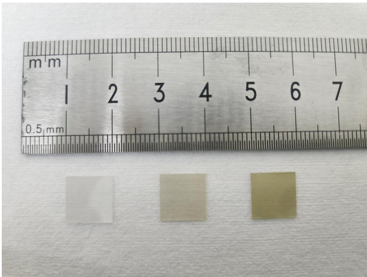
**Figure.S3** Photo of sapphire substrate(left), MoS<sub>2</sub> film after 50 cycles growth(middle), MoS<sub>2</sub> film after 100 cycles growth(right), showing that the ALD process is highly uniform and controllable.
