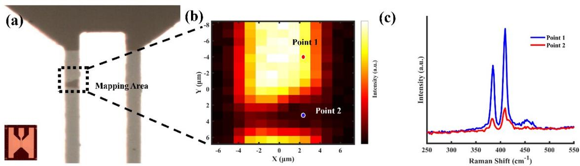
**Figure.S8** (a) Optical image of the filament area. (b) Raman mapping of the filament area. (c) Raman spectra of the polycrystalline film and the filament area. The weakening of the peaks indicates the breaking of the Mo-S bonds.
