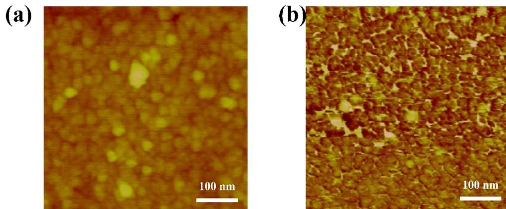
**Figure.S2** AFM images of the MoS<sub>2</sub> film (a) before and (b) after annealing. The amorphous clusters were transformed into a flake-like polycrystalline state.
