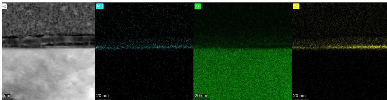
**Figure.S7** HR-TEM image and EDS mapping of the edge of the filament area. The disappearance of the oxygen content gap and the reduction in the S content indicate the oxidation process (right side: pristine film; left side: filament area).
