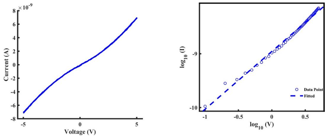
**Figure.S6** (a)  $I$ - $V$  curve of the device before electroforming and (b) log-log fitting of the curve. The slope of dotted line is 1.04, which indicates ohmic conduction in the pristine film.
