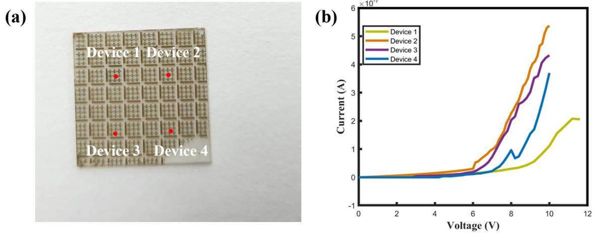
**Figure.S4** Electroforming process characteristics of four independent devices.. (a) Photo of the devices (b) Electroforming process. The threshold voltage ranged from 6 V to 9 V, indicating that the electroforming process is commonly observed.
