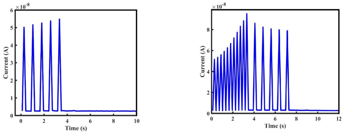
**Figure.S12** Current responses to consecutive pulses after the device has been subjected to pulses at different frequencies. (a) Potentiation caused by five consecutive pulses (8 V, width of 0.2 s, interval of 0.6 s). (b) Depression caused by a second group of five consecutive pulses (8 V, width of 0.2 s, interval of 0.6 s) following the first five consecutive pulses (8 V, width of 0.2 s, interval of 0.1 s).
