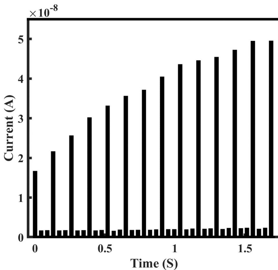
**Figure.S10** Current changes during positive pulse potentiation. The magnitudes and widths of the stimulation pulses and the read pulses were set at 5 V/50 ms and 1 V/50 ms, respectively. The time interval between pulses was 50 ms. The power consumption of each set pulse/read pulse is lower than 0.25  $\mu$ W/2 nW, respectively.
