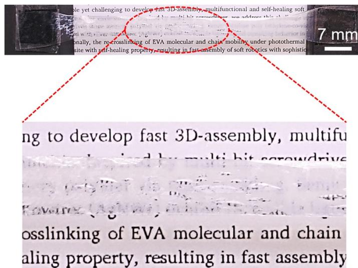
Fig. S2 An inhomogeneous composite film from the casting method.
