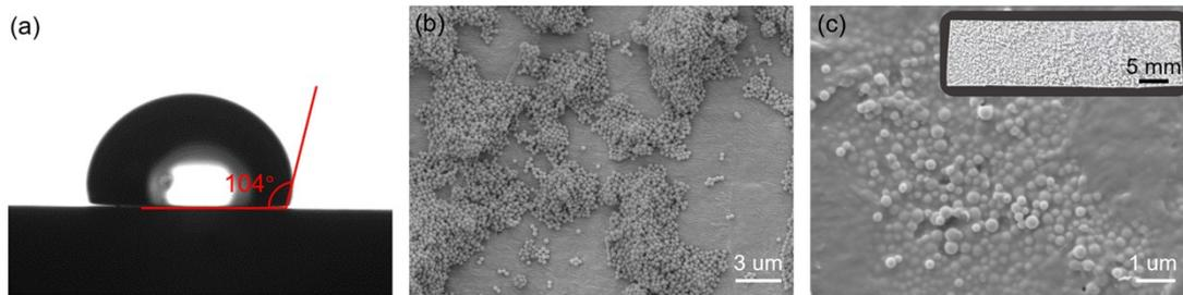
Fig. S1 (a) Water contact angle of PI substrate without fluorination. (b) SiO<sub>2</sub> NPs are left on PI substrate without fluorination. (c) SEM image and digital photo of complex film peeled off the un-fluorinated PI substrate.
