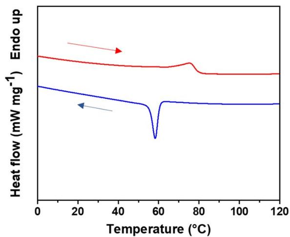
Fig. S5 DSC second heating and cooling curves of SiO<sub>2</sub>/EVA composite films.
