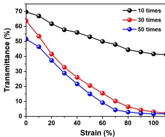
Fig. S8 Transmittance at wavelength of 750 nm of SiO<sub>2</sub>/EVA composite films versus NPs spray times as a function of applied strain.
