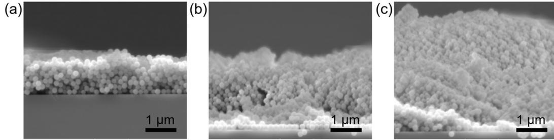
Fig. S6 Cross-sectional SEM images of SiO<sub>2</sub> layer with different spray times, (a) 10 times, (b) 30 times, (c) 50 times.
