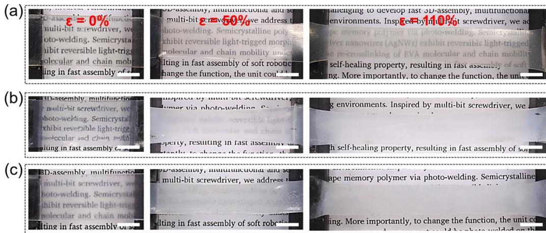
Fig. S7 Optical images of SiO<sub>2</sub>/EVA composite films with different spray times, (a) 10 times, (b) 30 times, (c) 50 times at specific strains. Scale bar: 5 mm.
