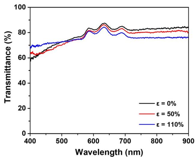
Fig. S4 Transmittance spectra of crosslinked EVA film without SiO<sub>2</sub> NPs upon stretching.
