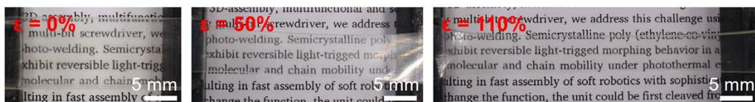
Fig. S3 Optical images of crosslinked EVA film without SiO<sub>2</sub> NPs at specific strains.
