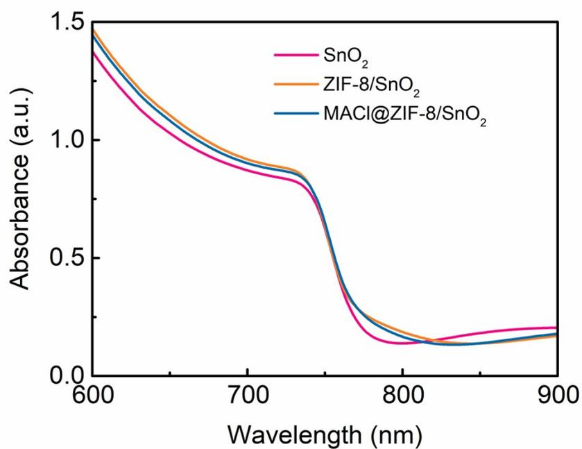
**Fig. S4** UV-vis absorbance spectra of the perovskite films based on different ETLs.
