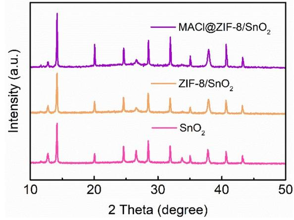
**Fig. S5** XRD patterns of perovskite films based on different ETLs.
