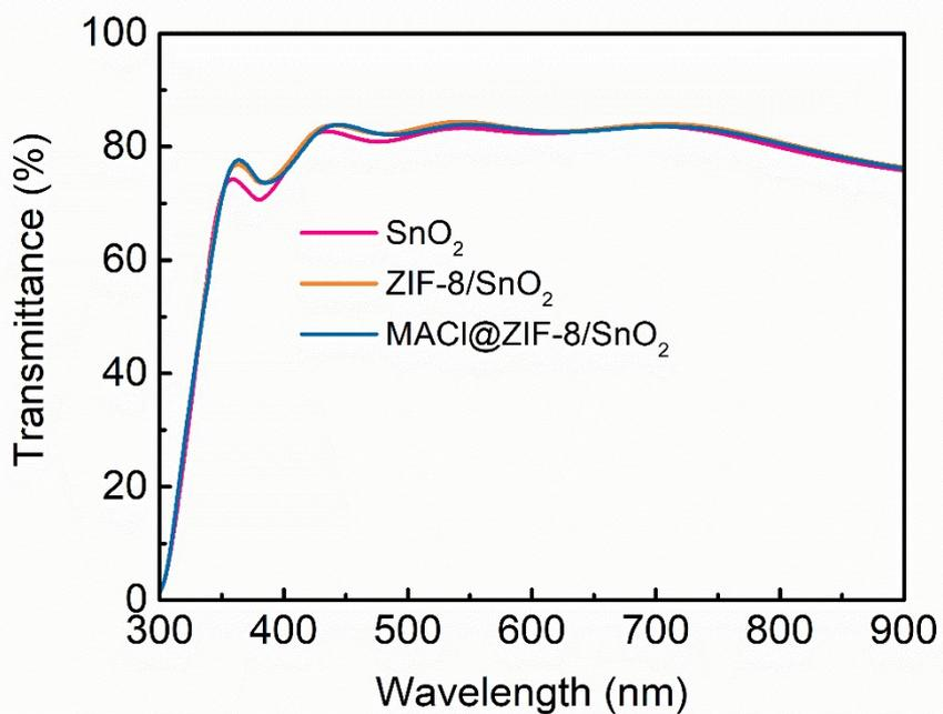
**Fig. S2** UV-vis transmittance spectra of the different ETLs.
