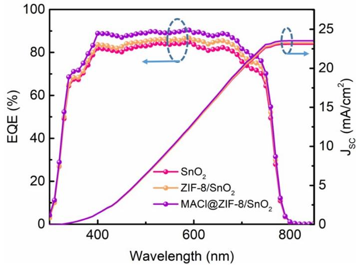
**Fig. S7** EQE curves of devices based on SnO<sub>2</sub>, ZIF-8/SnO<sub>2</sub>, and MACl@ZIF-8/SnO<sub>2</sub>, respectively.
