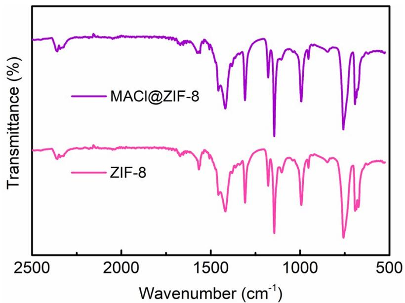
**Fig. S1** FTIR spectra of ZIF-8 and MACl@ZIF-8.
