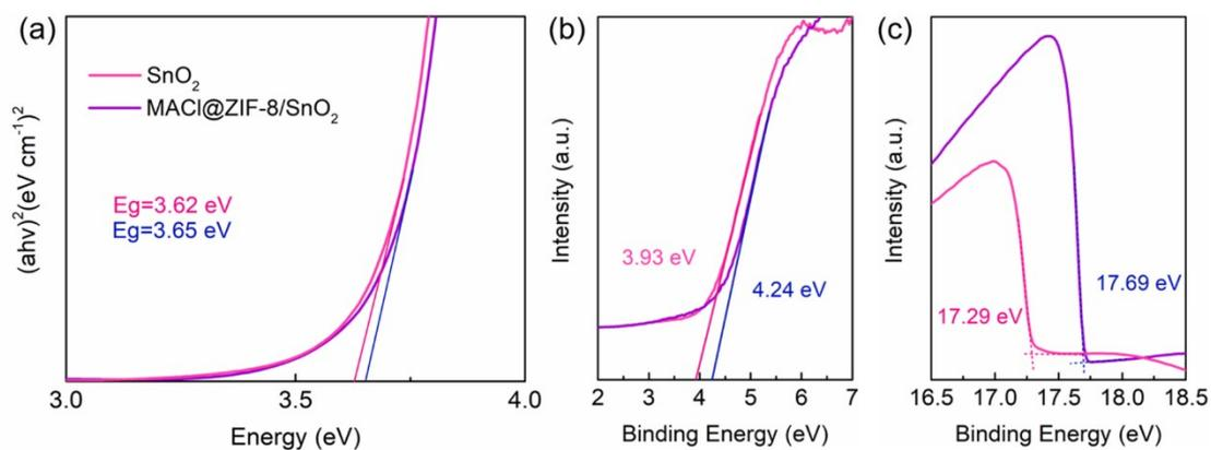
**Fig. S3** (a) Tauc plots calculated from UV-vis spectra. (c) Valence regions in UPS survey and (b) secondary-electron cutoff spectra.
