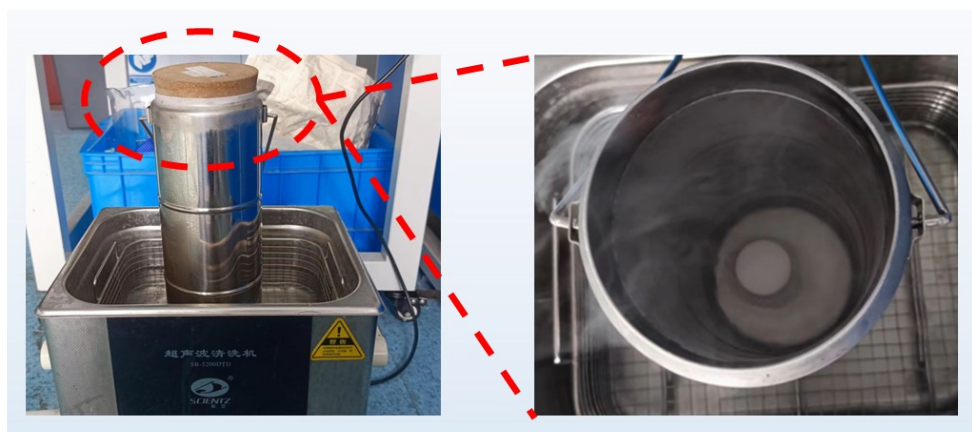
Fig S1. Photos of the setup of the ultrasonic-assisted liquid nitrogen freezing process.
