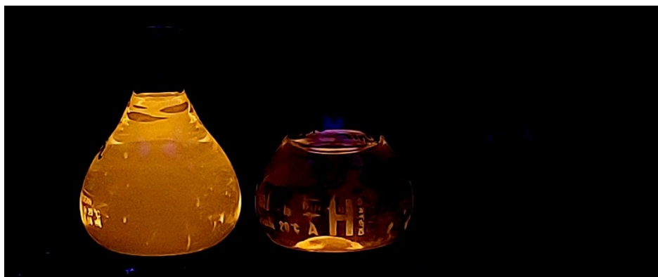
Figure S22. Emission of BPN in toluene, THF and dichloromethane (from left to right) ( c = 10^{-4} mol/L, \lambda_{exc} = 365 nm).
