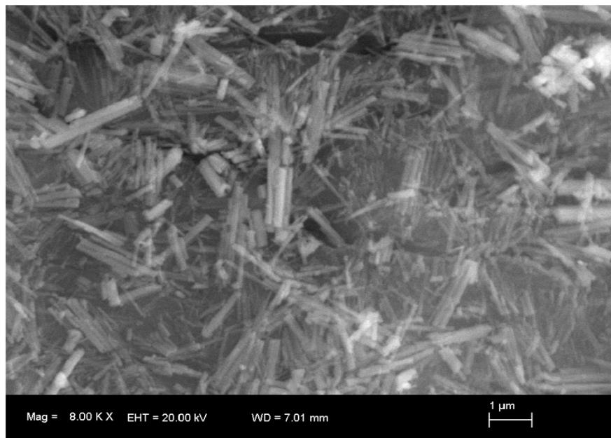
**Figure S1.** SEM images of  $\text{NaYF}_4$ :  $\text{Gd}^{3+}$ ,  $\text{Yb}^{3+}$ ,  $\text{Er}^{3+}$  nanoparticles crystallizing in rod-shape.
