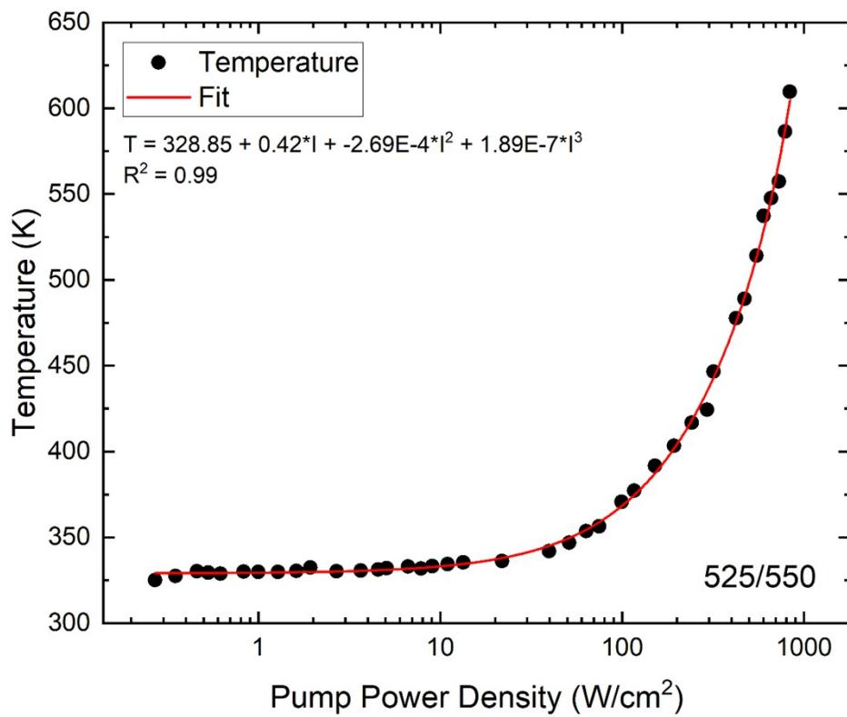
**Figure S2.** Relation between temperature and pump power density on the sample, obtained by the ratio between the LIR (525/550nm) and temperature.
