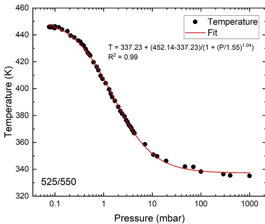
**Figure S3.** Relation between temperature and pressure on the sample, obtained by the ratio between the LIR (525/550nm) and temperature.
